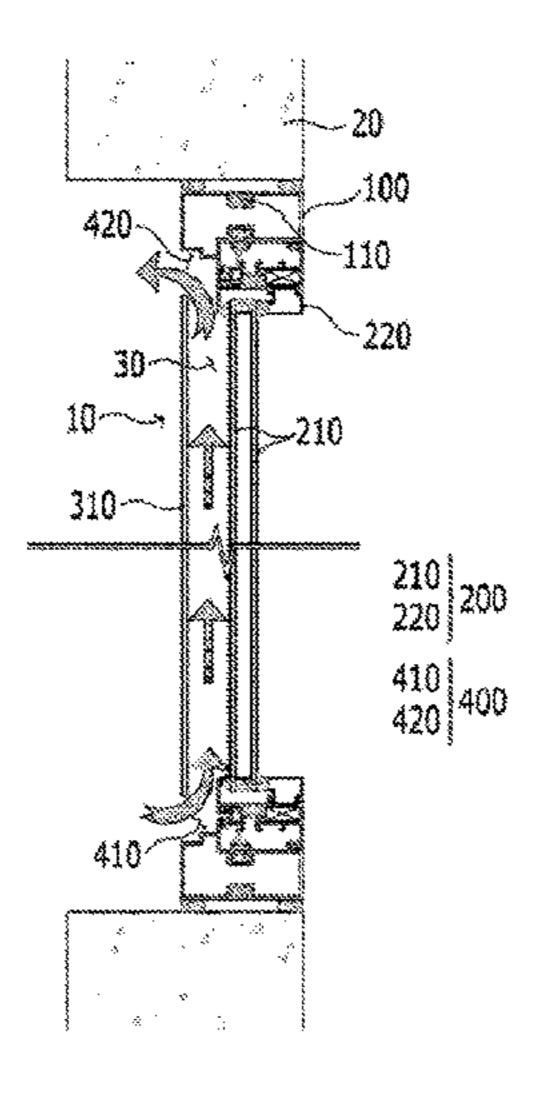
window; an air-flowing opening formed between the outer window and the window frame to form a flow path in which air in the hollow layer flows or circulates; and an opening and closing device provided at one side of the inner window to open and close the inner window from the window frame. The outer window may include a tinted glass or a glass having a high absorption rate and a bracket for fixing the tinted glass to the window frame.
