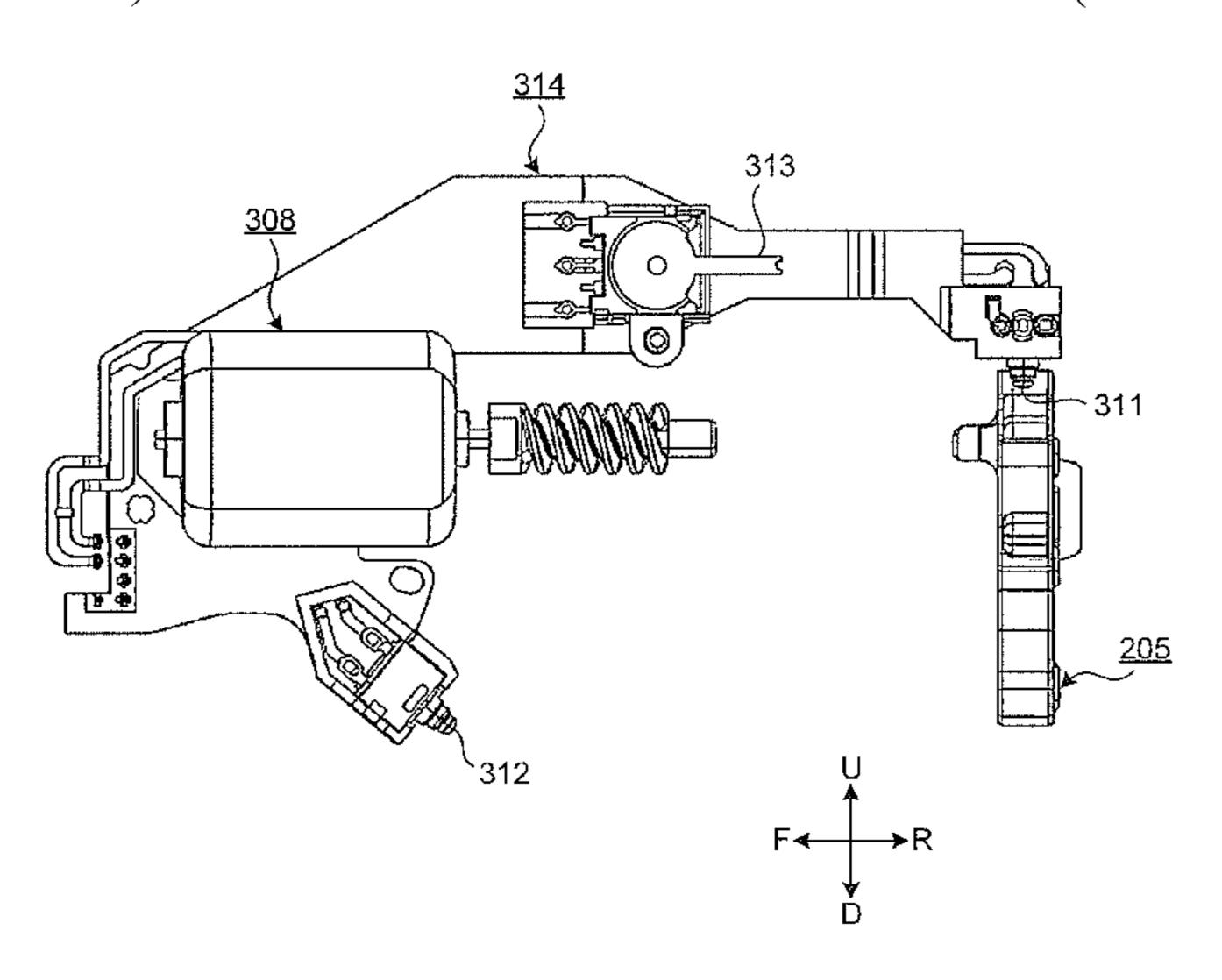
half closed door detection switch having a switch pin configured to abut against the latch. A plane of rotation of the latch and a plate surface of the switch plate intersect each other orthogonally.
