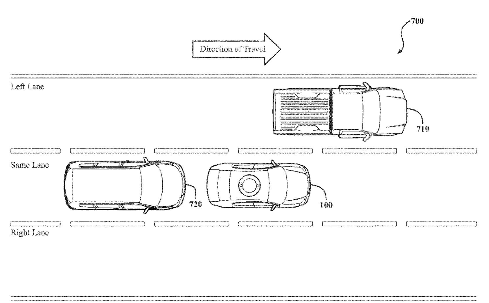
generating prediction indicators for the nearby vehicles as a function of the factors for the lanes using the S-RNN. The method includes providing electronic outputs identifying the prediction indicators that specify a likelihood of the nearby vehicles changing between the lanes.
