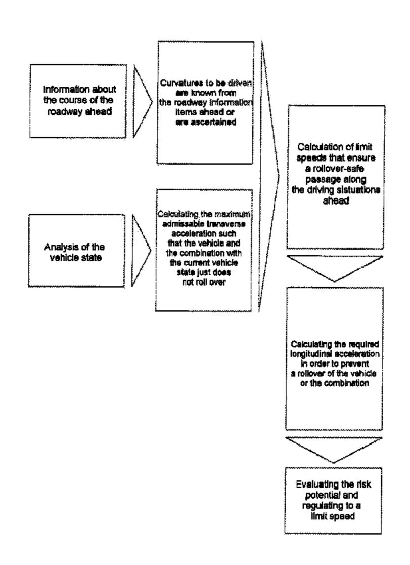
the current load of the vehicle or the tractor-trailer combination. Also described is a related apparatus for preventing a rollover of a vehicle or a tractor-trailer combination in curves.
