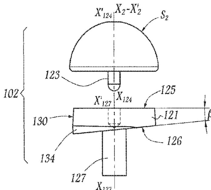
A surgeon can select the component in which the axes of symmetry of the components are oriented differently with respect to their rear faces.
