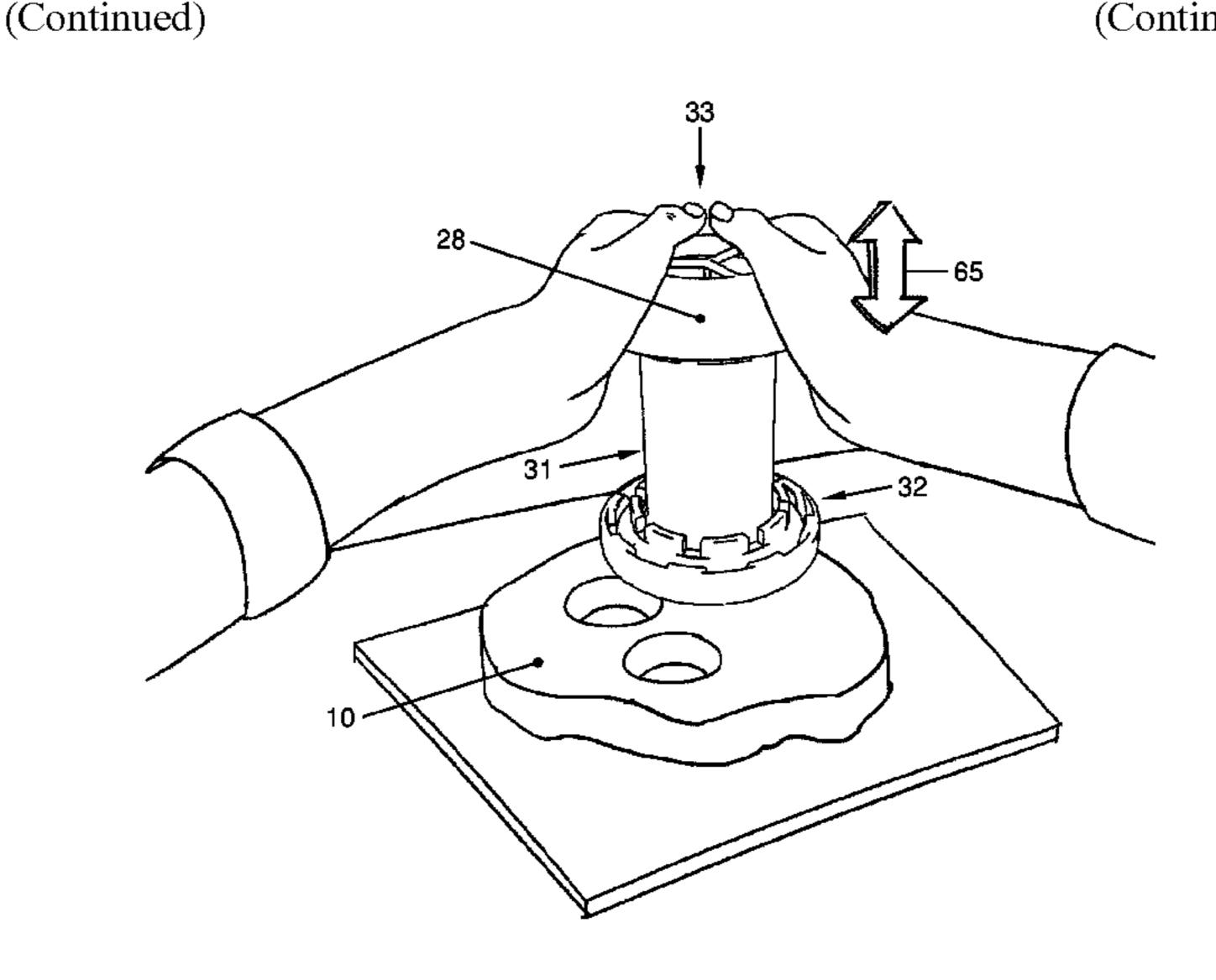
for automatically inserting said punched slices into the inner space of the cartridge. Thanks to this punch-fill connector the manual (re)filling of the cartridge can be performed more easily and more reliably.
