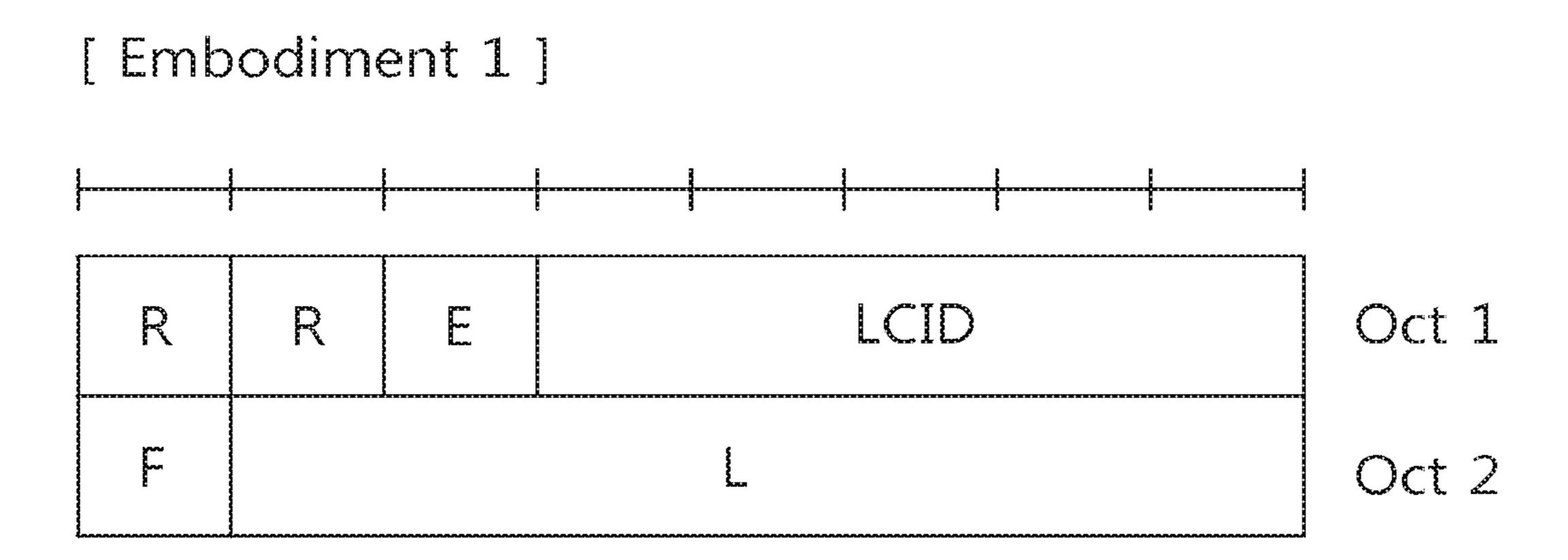
R/R/E/LCID/F/L sub-header with 7-bit L field
