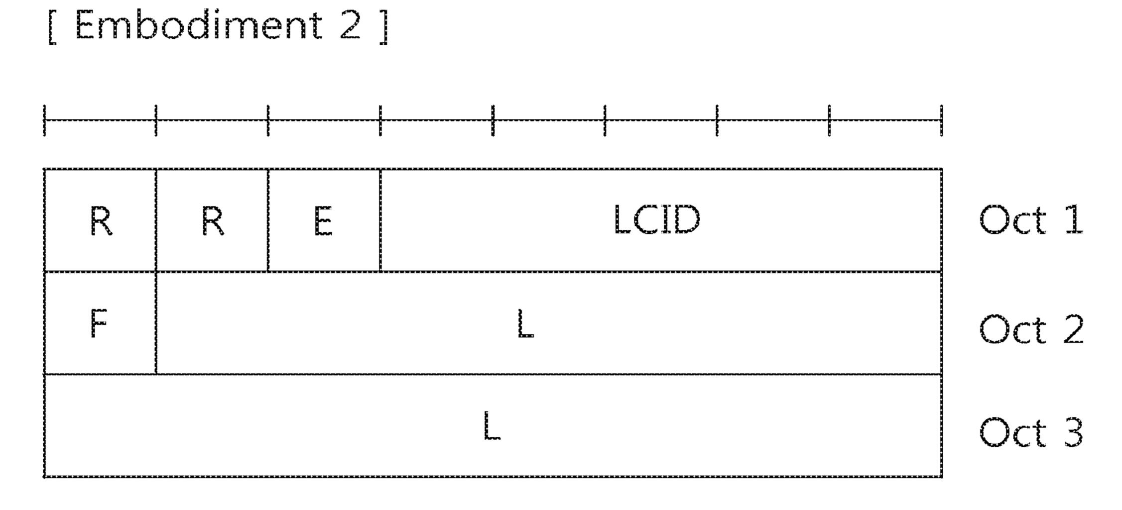
R/R/E/LCID/F/L sub-header with 15-bit L field
