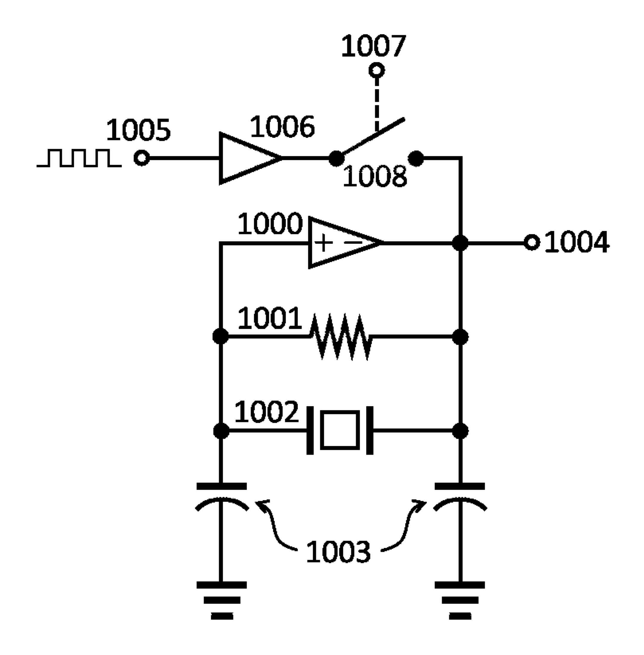
**Figure 11** (Embodiment of the present invention, at which the start-up stimulus is realised as a time-variant current pattern)
