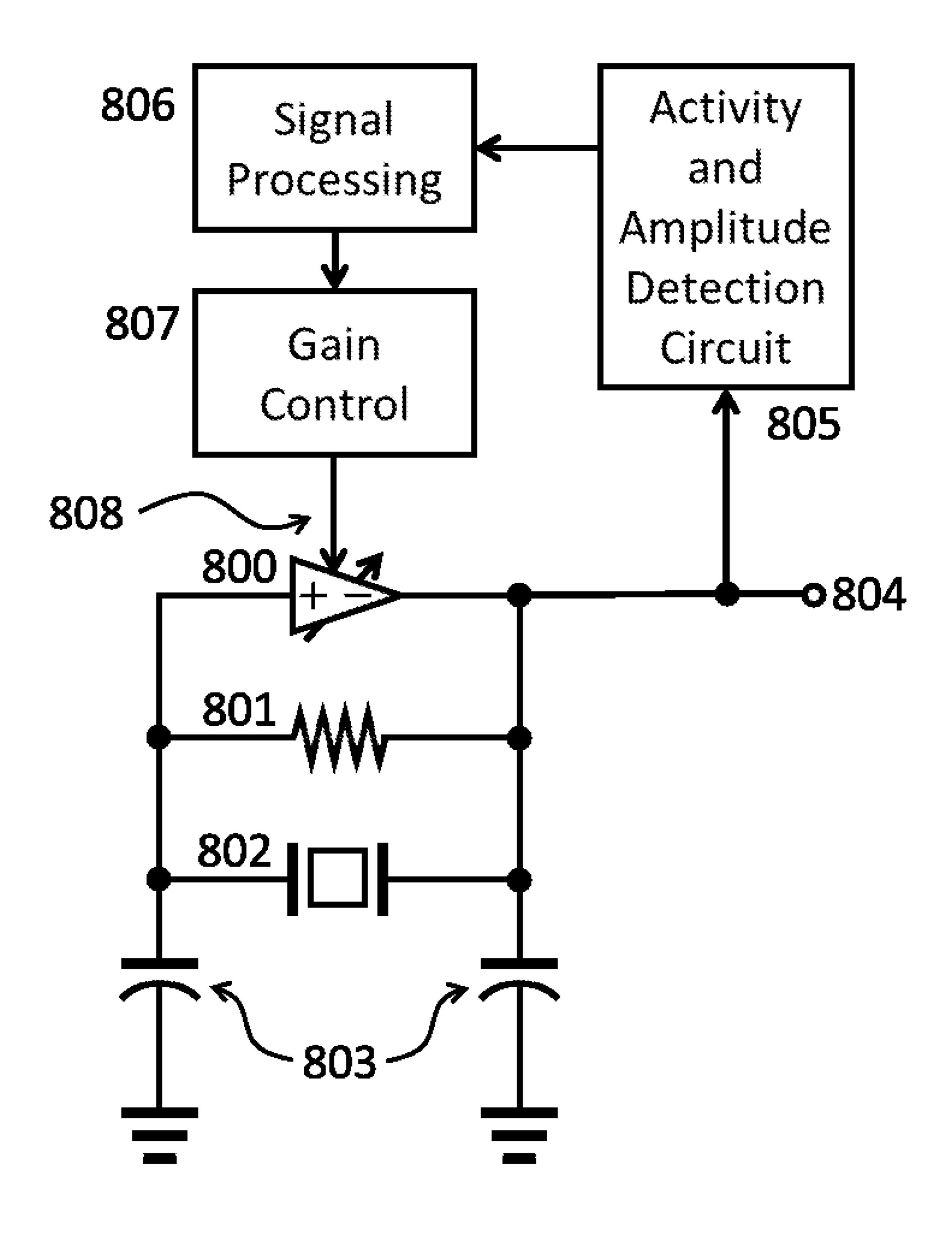
**Figure 9** (Schematic diagram of a crystal oscillator comprising a start-up shortening technique, according to prior art)
