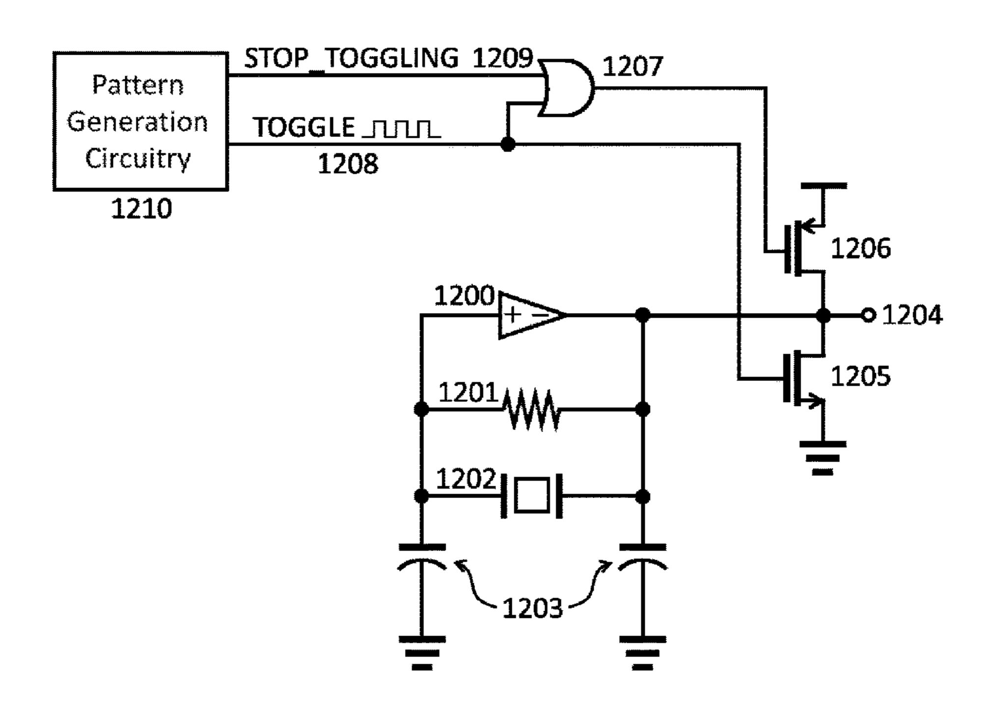
Figure 1 (Schematic diagram of the Pierce crystal oscillator, according to prior art)
