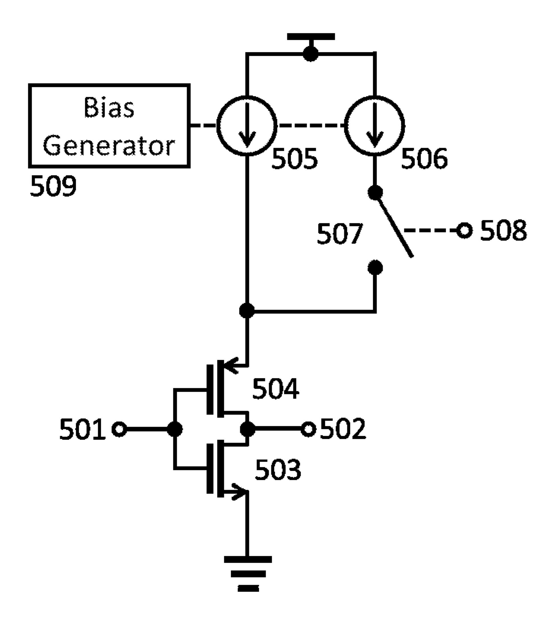
Figure 6 (Schematic diagram of a crystal oscillator comprising a start-up shortening technique, according to prior art)
