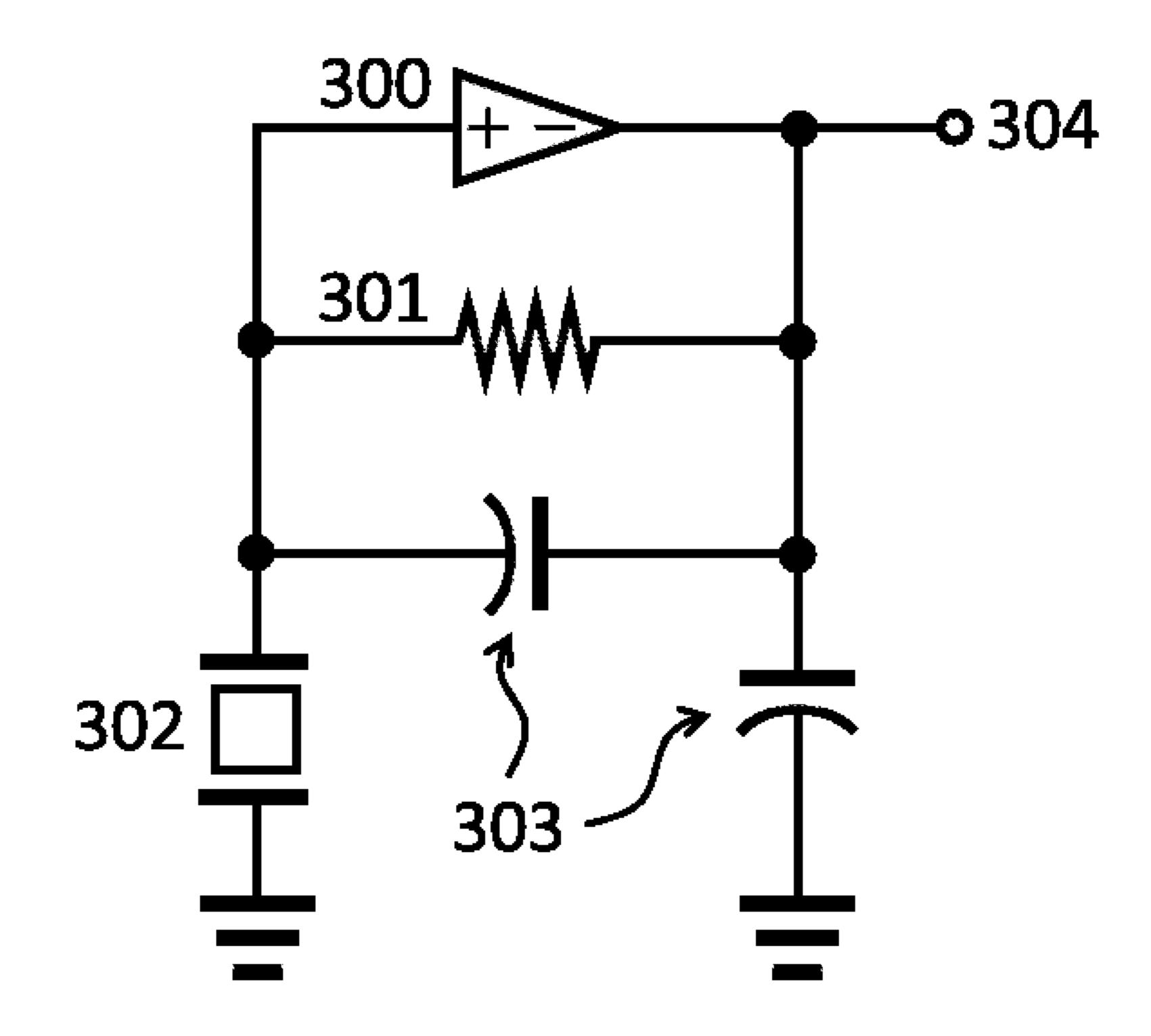
**Figure 4** (Schematic diagram of a crystal oscillator comprising a start-up shortening technique, according to prior art)
