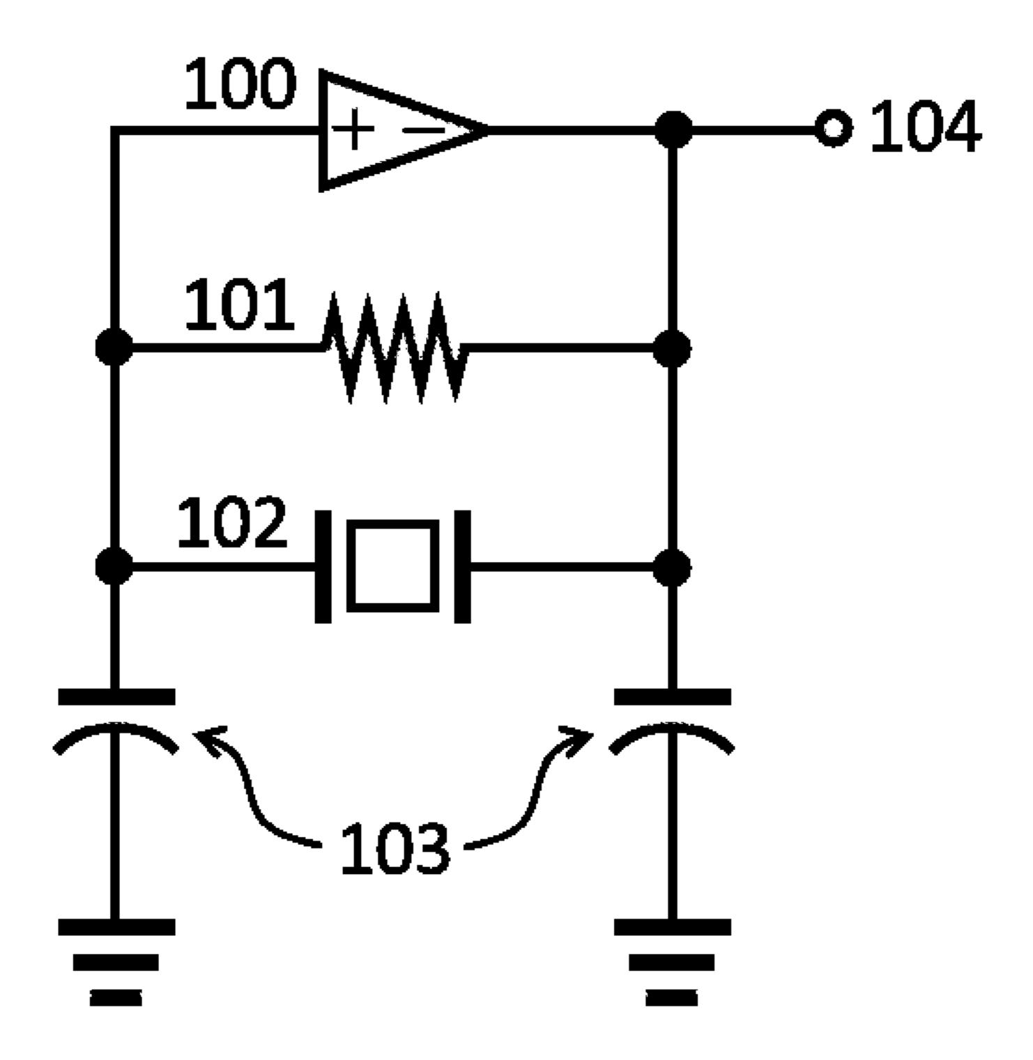
Figure 2 (Schematic diagram of the Colpitts crystal oscillator, according to prior art)
