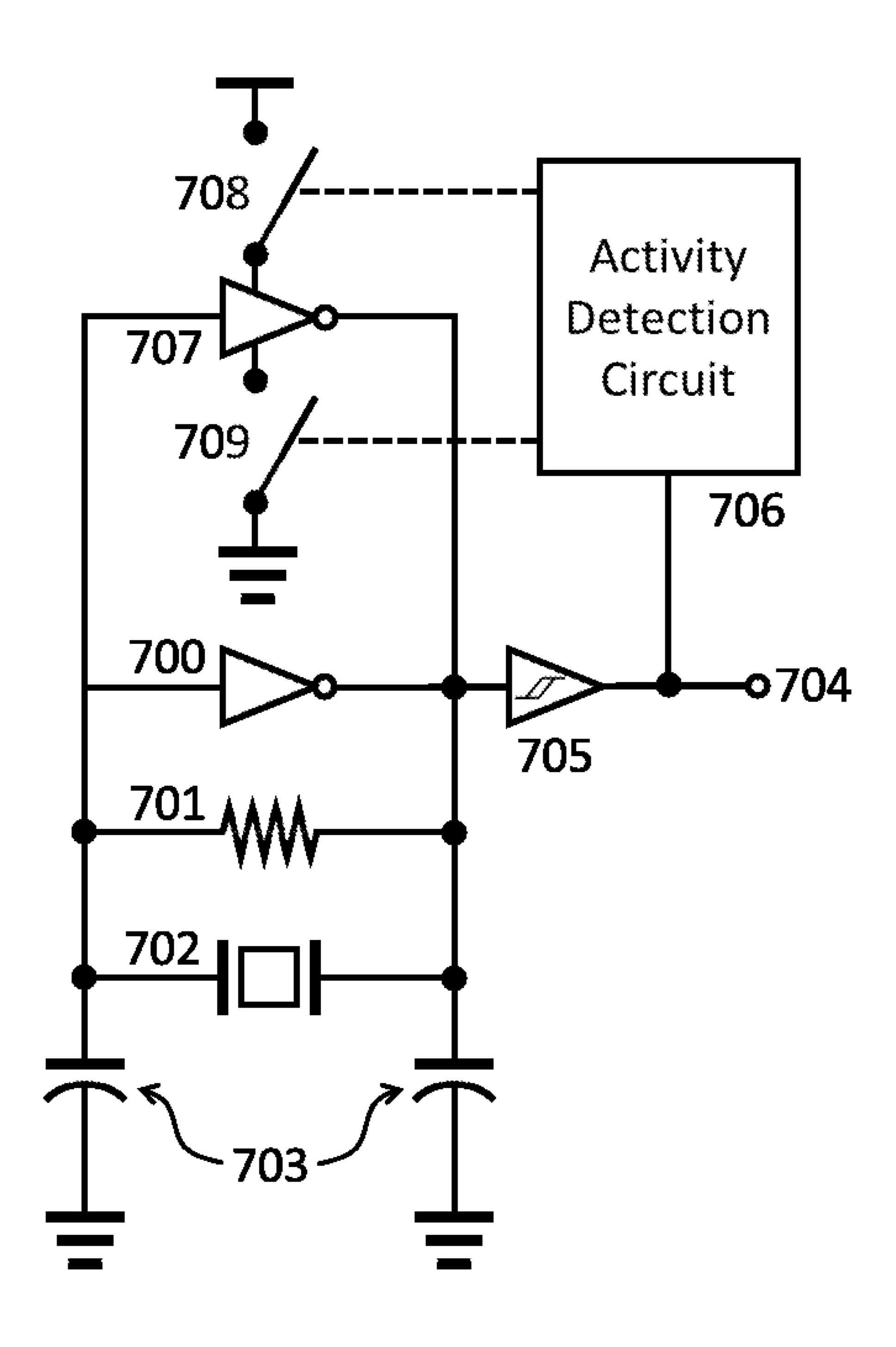
**Figure 8** (Schematic diagram of a crystal oscillator comprising a start-up shortening technique, according to prior art)
