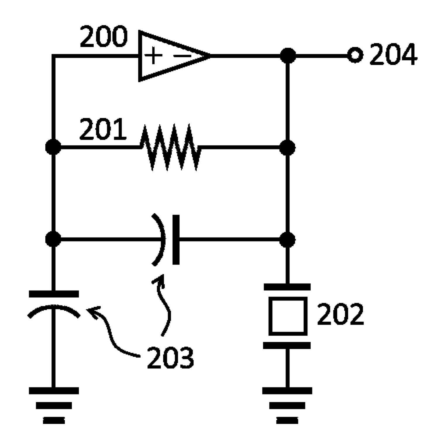
Figure 3 (Schematic diagram of the Santos crystal oscillator, according to prior art)
