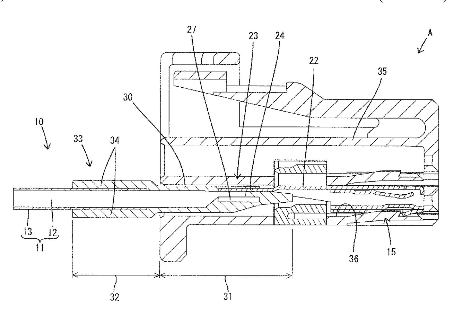
(30) covering the entire exposed area of the core (12) including a crimped part to the barrel (23) in a liquid-tight manner. A front end of the core (12) is disposed behind those of the crimping pieces (27). The barrel (23) is formed with a communicating portion (29) for causing a crimping space (28) of the barrel (23) to be open in an outer peripheral surface of the barrel (23) on a side before the front end of the core (12).
