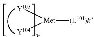
wherein Met is a metal; (Y<sup>103</sup>-Y<sup>104</sup>) is a bidentate ligand, Y<sup>103</sup> and Y<sup>104</sup> are independently selected from C, N, O, P, and S; L<sup>101</sup> is another ligand; k' is an integer value from 1 to the maximum number of ligands that may be attached to the metal; and k'+k'' is the maximum number of ligands that may be attached to the metal.
