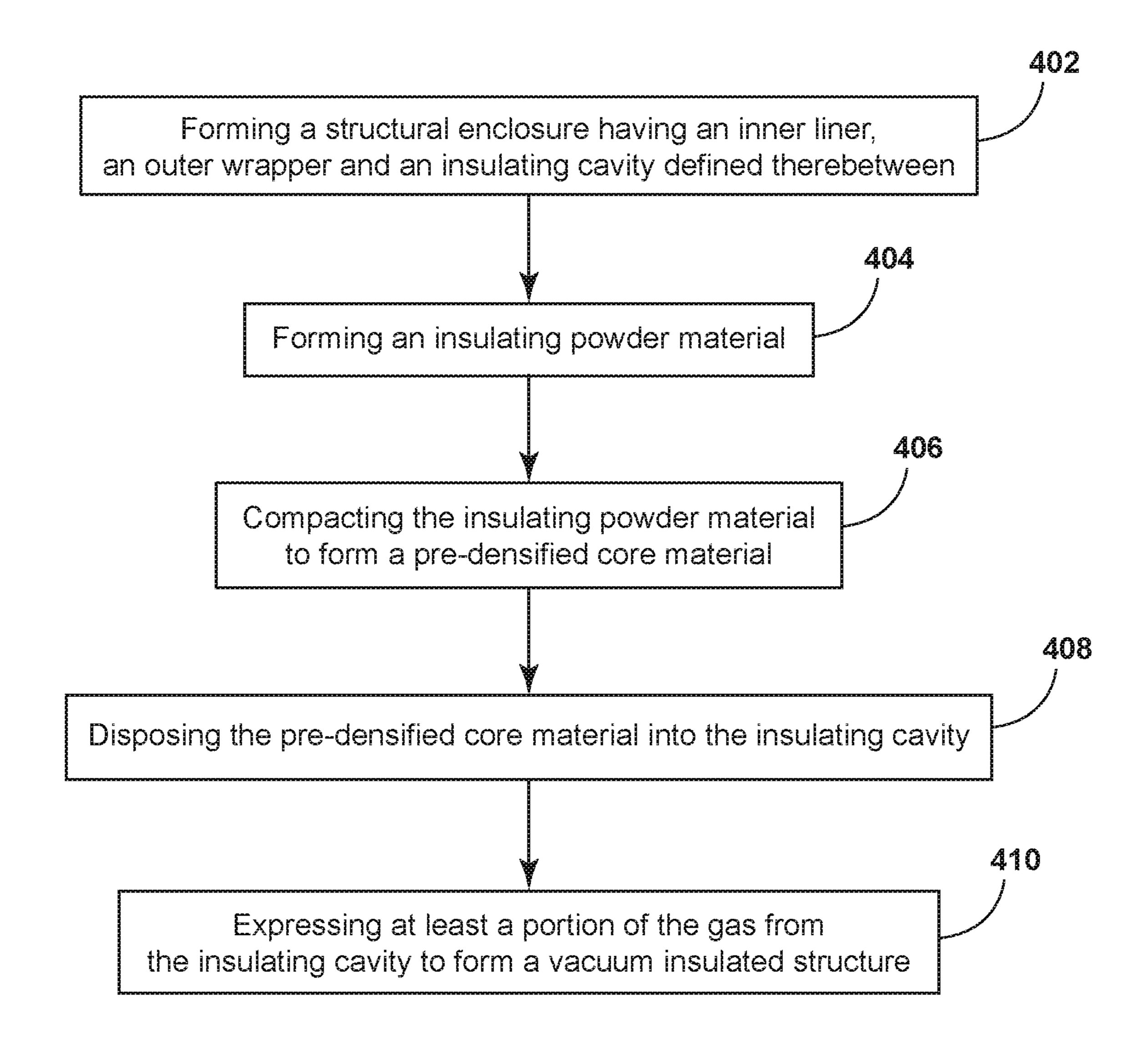
Method 600 for Forming an Insulated Structure for an Appliance
