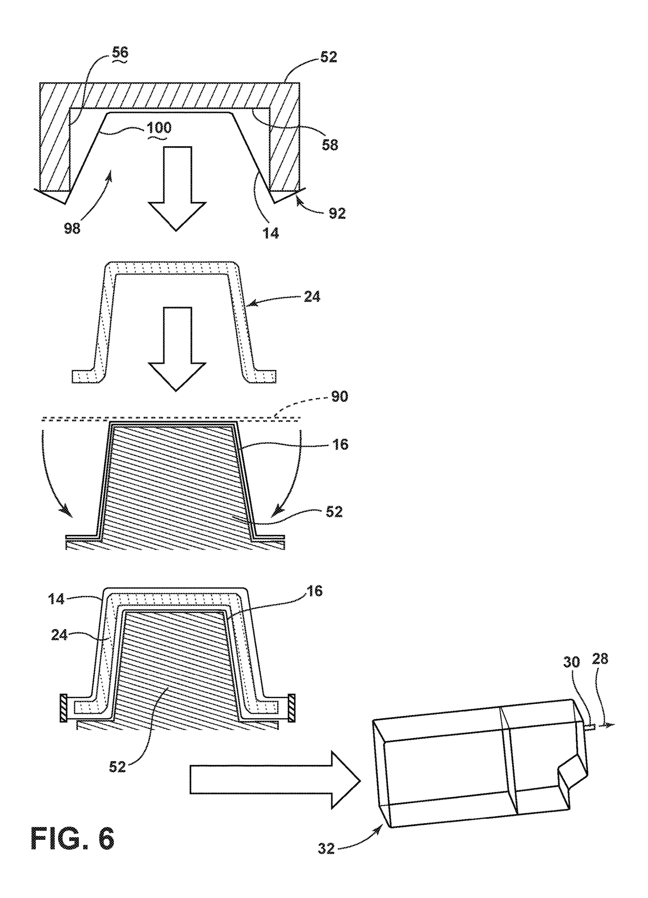
Method 400 for Forming an Insulated Structure for an Appliance
