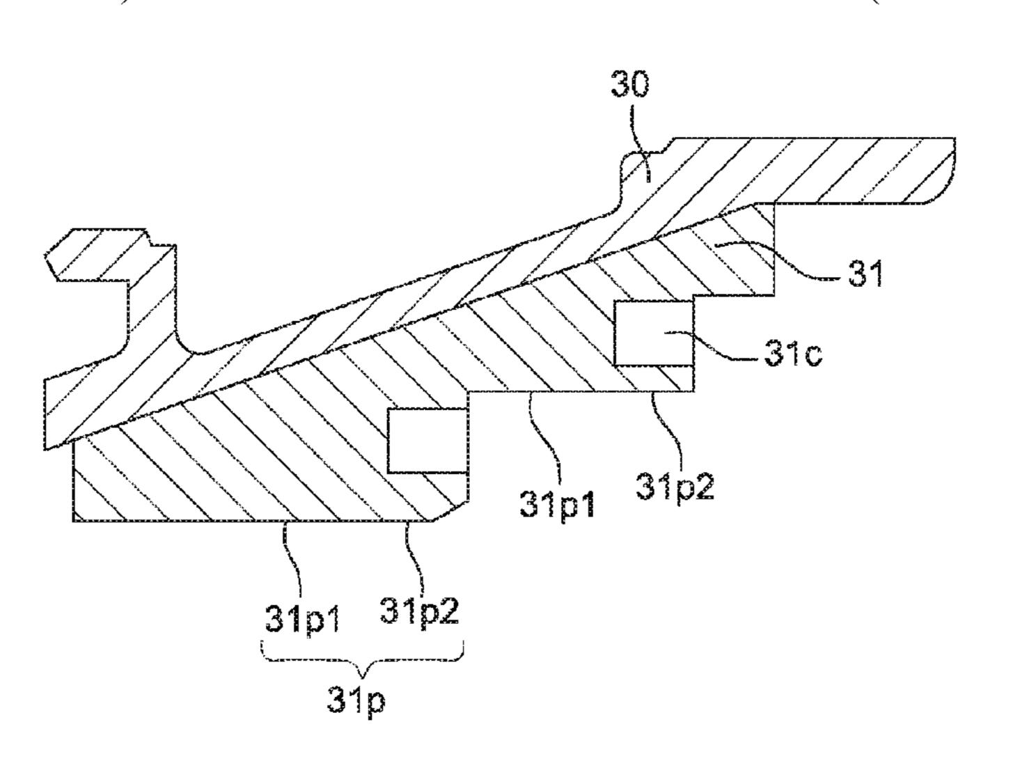
axial position of the wiper during nominal operation of the turbine, and a second area adjacent to the first area and having lower wiper penetration resistance than the first area. The second area is located downstream from the first area and corresponds to the axial position that the wiper takes when a flame goes out in the combustion chamber of the engine.
