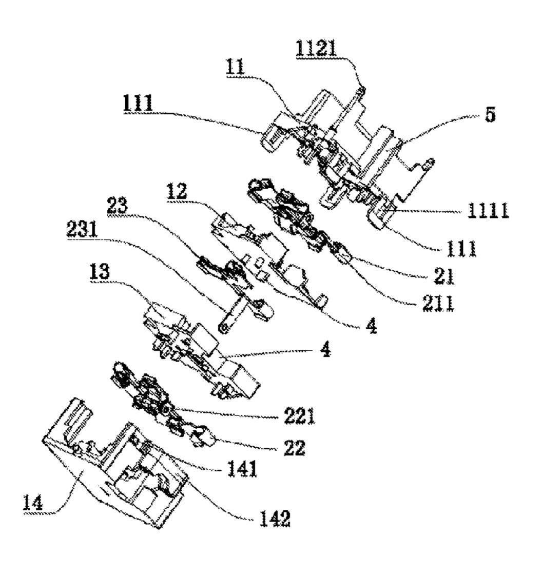
is corresponding to the live wire plug bush conductive sheet, the naught wire plug bush conductive sheet and the earth wire plug bush conductive sheet.
