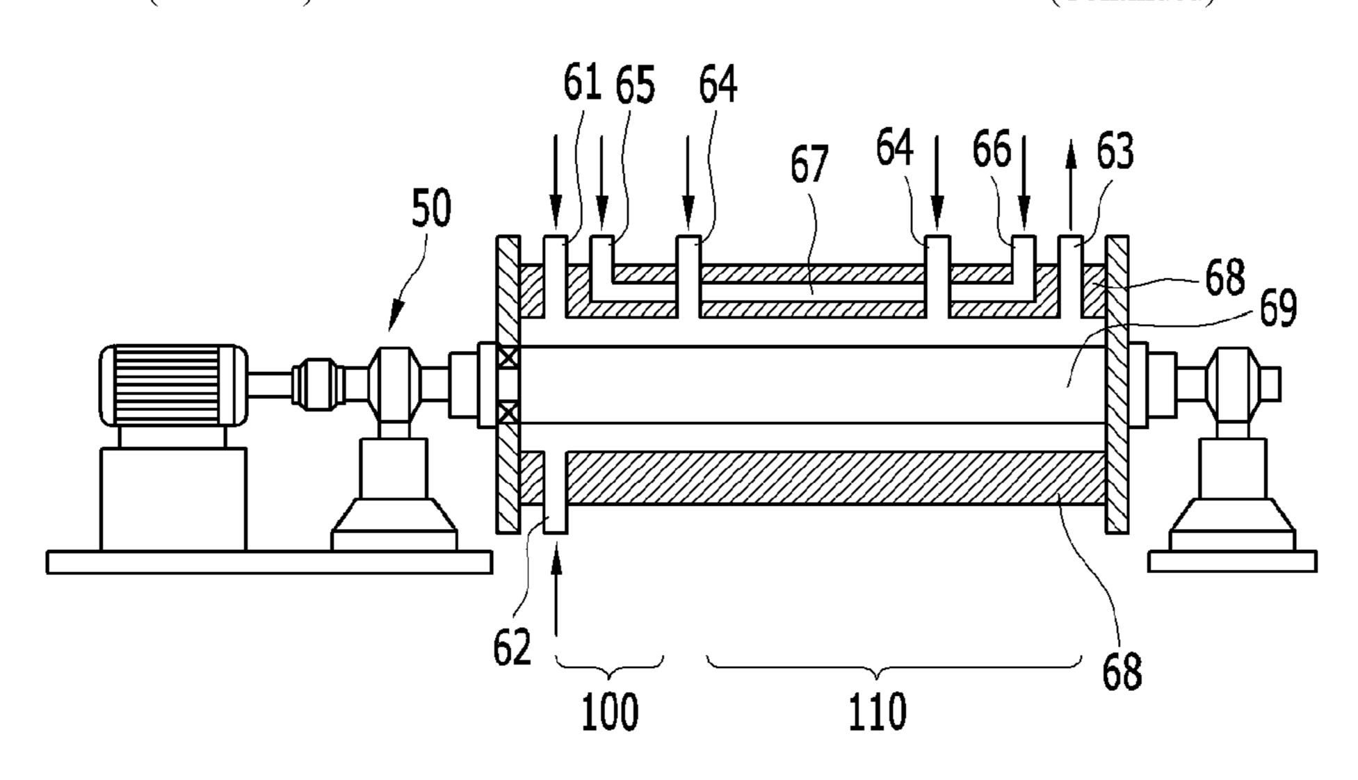
cylinder in which the rotor rotates; supplying a shell material for coating the core to the interior of the cylinder in which a core-type precursor is formed; separating a liquid comprising core-shell particles formed through the supplying into a solid and a liquid; and drying the core-shell particles obtained through the separating.
