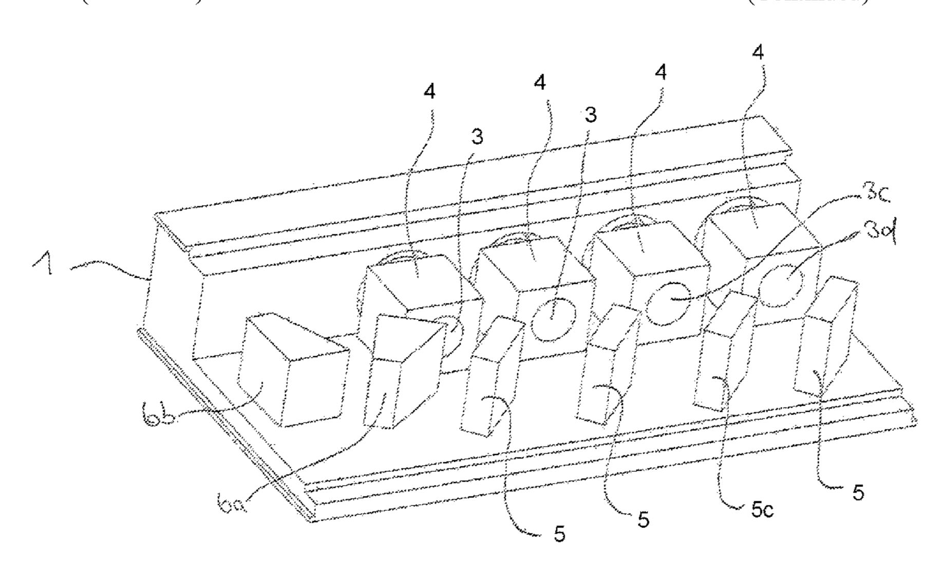
mating lenses (3) are disposed in a positioning module (4) that allows the collimating lenses (3) to be placed in different positions during the manufacturing process of the apparatus.
