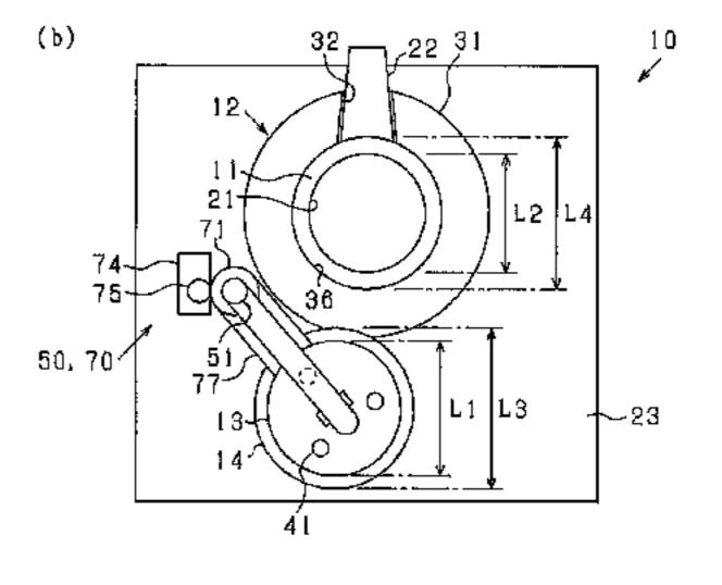
crucible, the first furnace lid is removed from the opening, and the second furnace lid is disposed in the position in which the opening is closed.
