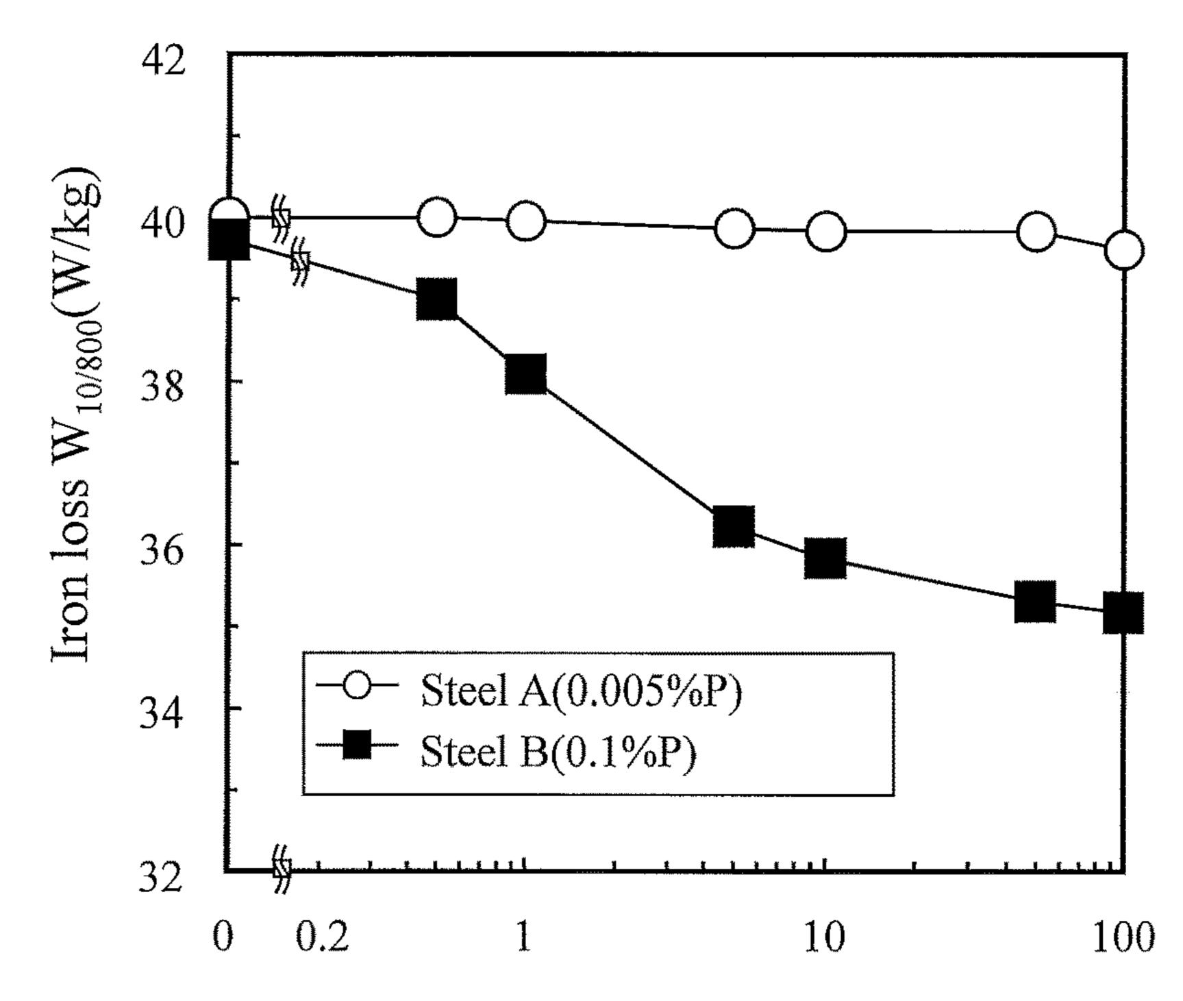
Heat treating time after finishing annealing (hr)
