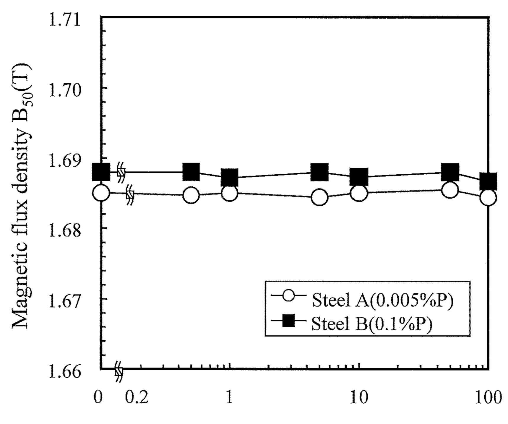
Heat treating time after finishing annealing (hr)
