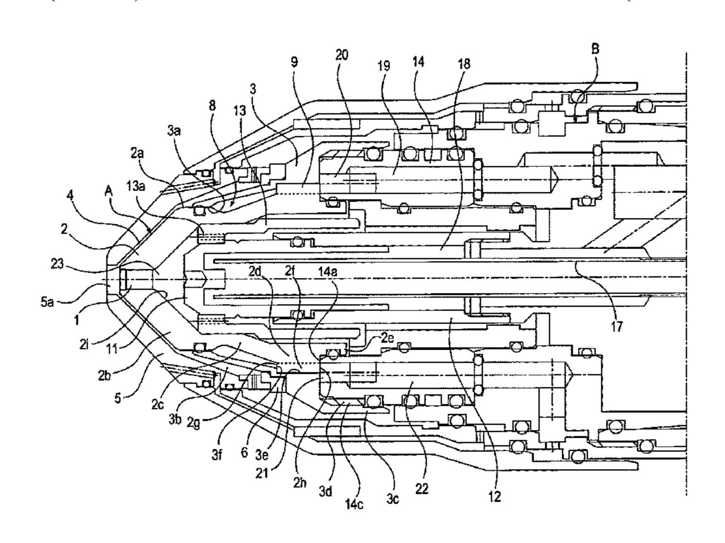
a groove extending on a plane crossing the axis and is connected to the water passage. When the nozzle is fastened to the torch body, one of the independent water passages communicates with the water supply port and another communicates with the water drain port. Rear end surface of inner nozzle is in contact with end surface of the nozzle base thereby obtaining electrical conductivity.
