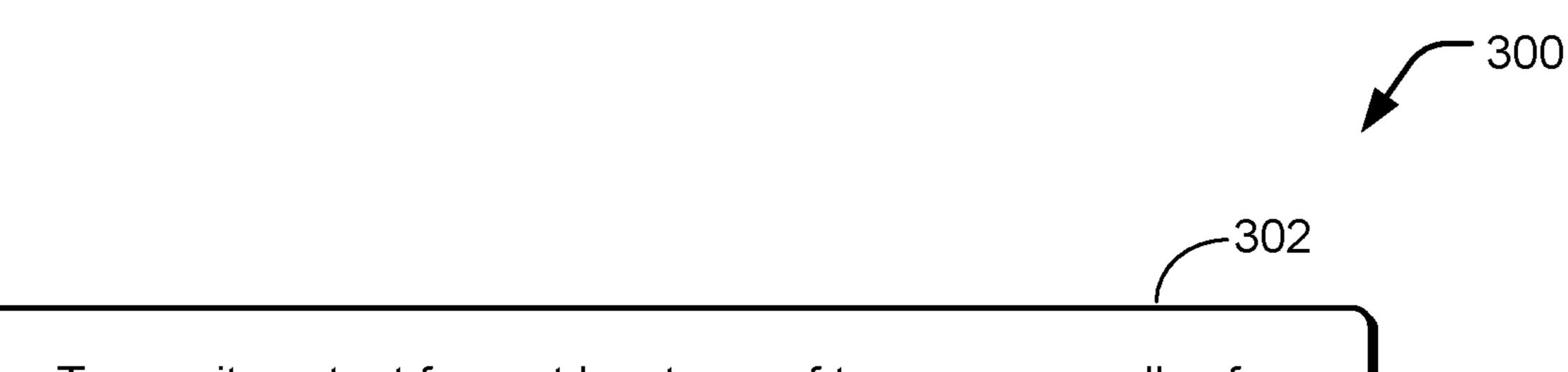
Transmit content from at least one of two or more cells of a wireless communication network to a plurality of user devices in a predetermined geographic area over one or more dedicated downlink channels as a multimedia broadcast multicast service
