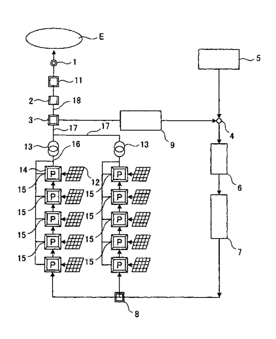
basis of a power generation level setting value demanded by an information processing unit, the instantaneous power detected by the instantaneous power detector (3) is controlled to be the target value set by the generated power setting unit (5).
