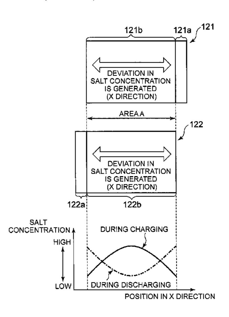
ture of the secondary battery. The controller is configured to calculate a salt concentration distribution in the power generation element based on the first flow velocity and the second flow velocity.
