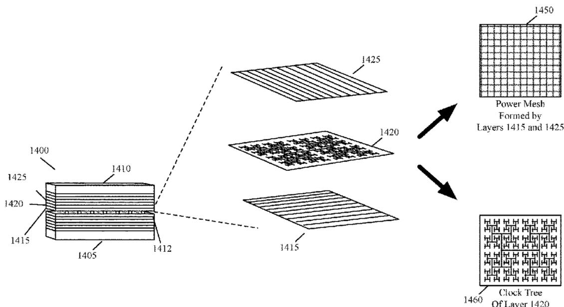
each other. In some embodiments, a subset of one or more interconnect layers of the second set interconnect layers of the second die has interconnect wiring that carries power, clock and/or data-bus signals that are supplied to the first IC die.
