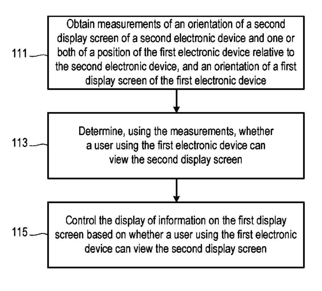
and controlling (105; 115) the display of information on the first display screen based on the result of the step of determining.
