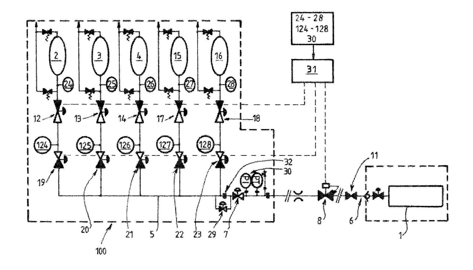
pressure regulation member, and a second isolation valve, the method comprising filling a first tank, characterized in that, on completion of the filling of the first tank and before filling a second tank, the first and second isolation valves are closed to trap a supply of pressurized gas in the circuit between said two valves and in that the supply of gas is used to refill at least one of the containers.
