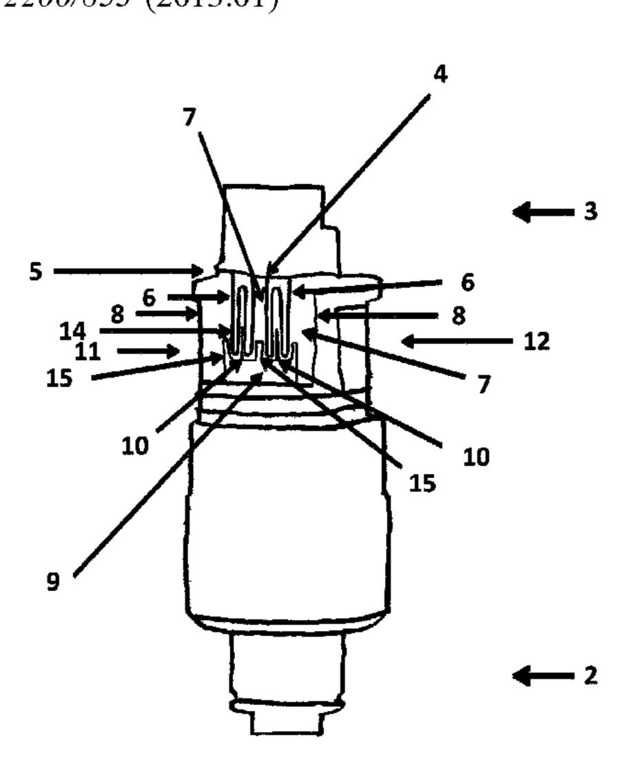
injector further comprises an overmolded body encapsulating the electrical connection between the base portion and the extension portion.
