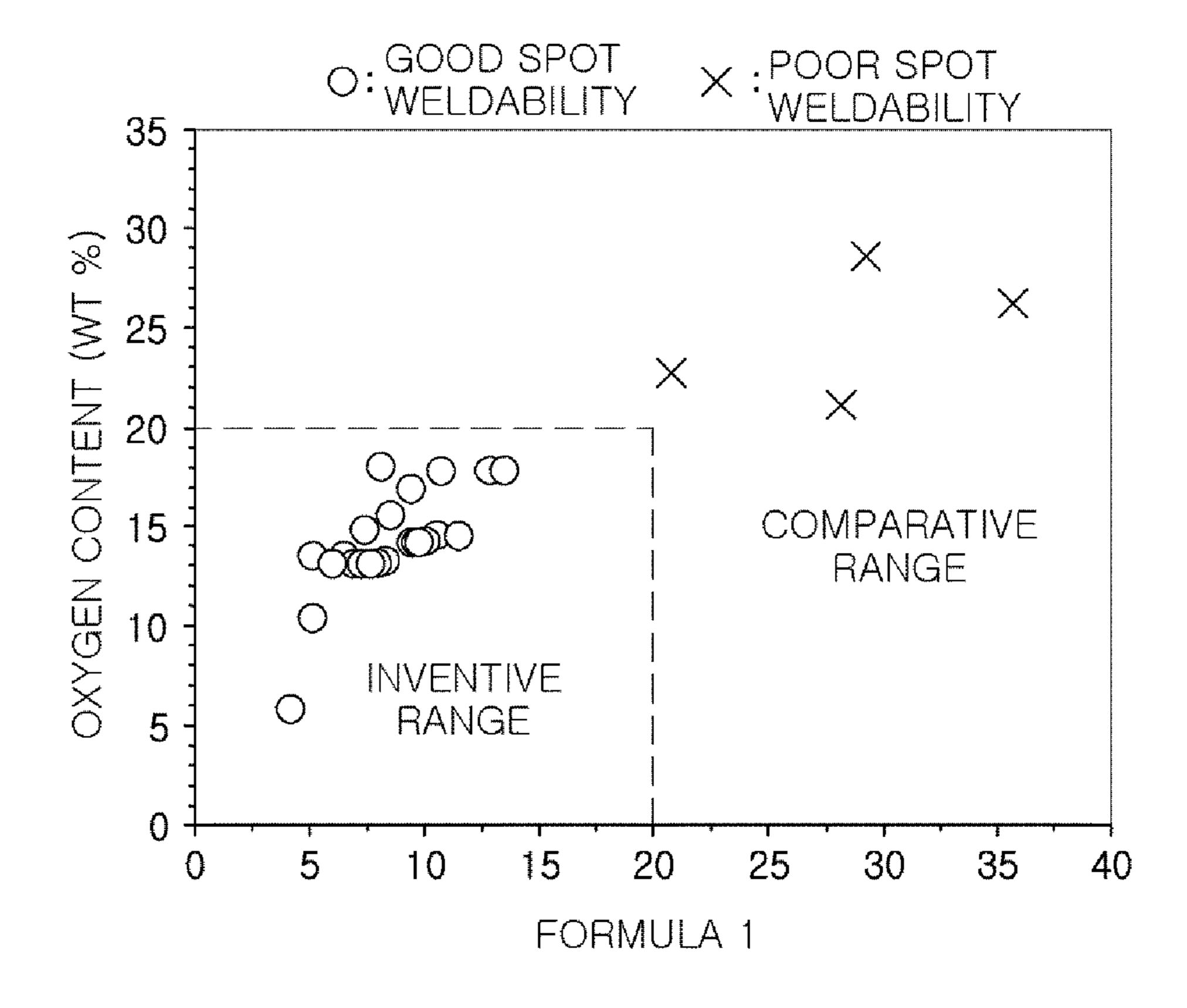
ALUMINUM-IRON ALLOY-COATED STEEL SHEET FOR HOT PRESS FORMING, HAVING EXCELLENT HYDROGEN DELAYED FRACTURE RESISTANCE, PEELING RESISTANCE, AND WELDABILITY AND HOT-FORMED MEMBER USING SAME
