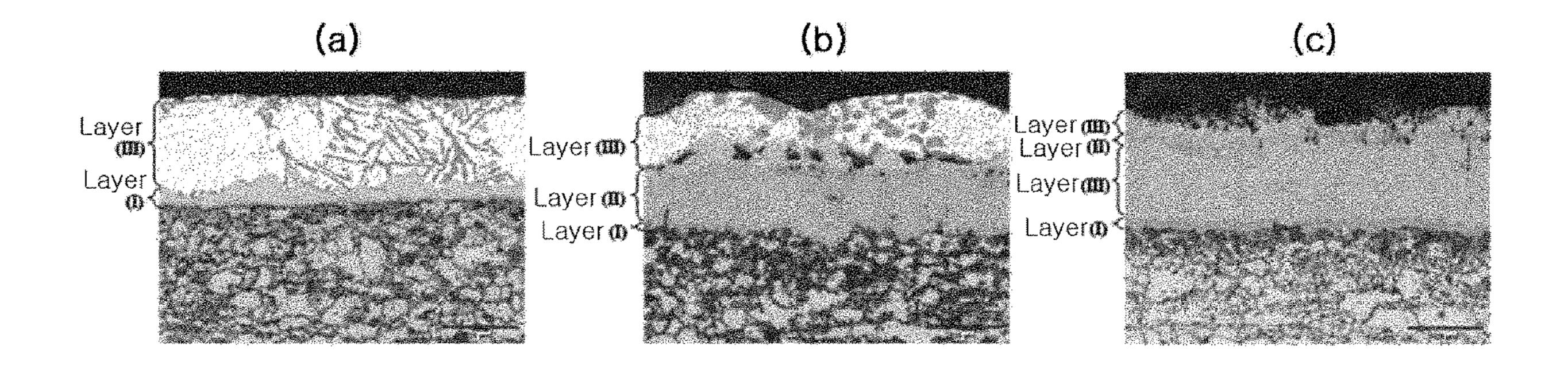
Al—Fe alloy layer II formed in the Al—Fe alloy layer III continuously or discontinuously in a length direction of the steel sheet, and having a Vickers hardness of 400~900 Hv, wherein an average oxygen content at a depth of 0.1 µm from a surface of the oxide layer is 20% or less by weight.
