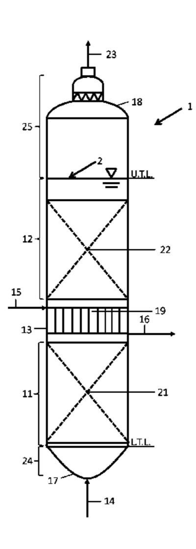
inlet conduit for feeding the gas mixture into the slurry bed, a filtration zone for separating the liquid hydrocarbons from the catalyst particles and a liquid outlet conduit for withdrawing the separated hydrocarbons from the filtration zone. The filtration zone is situated in the slurry bubble column reactor such that the slurry bed is found in a first and a second heat exchange zone with the filtration zone arranged between the first and the second heat exchange zone.
