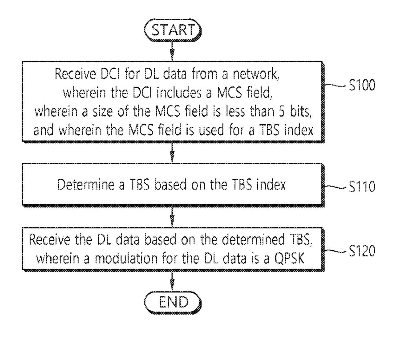
and the adapted code rate. The TBS may be determined based on a modulation and coding scheme (MCS) only.
