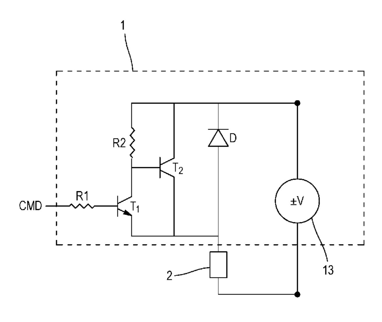
trical device (2); the switch (12) being sensitive to the discrete electrical control signal (CMD) for just one sense of voltage.
