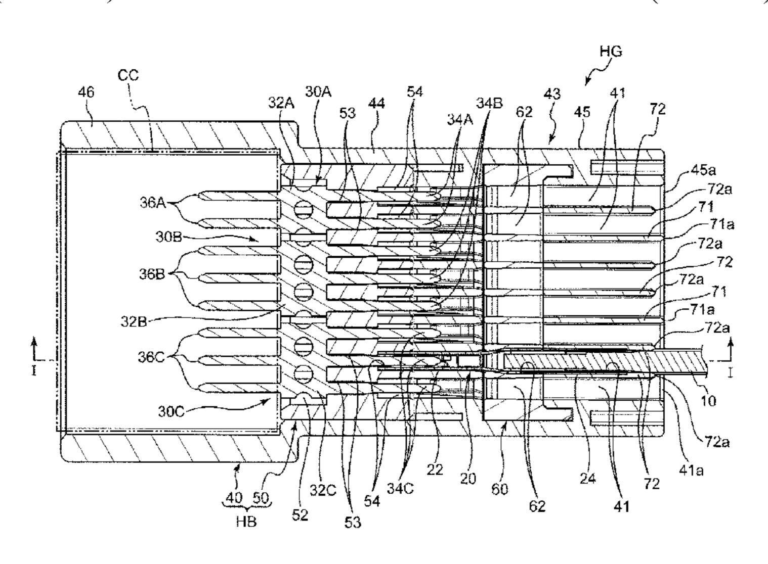
respectively accommodating the wire-side terminals to be insulated without being shorted to each other and second separation walls (72) interposed between the terminal accommodating chambers for respectively accommodating the wire-side terminals to be shorted to each other. The first and second separation walls (71, 72) are shaped so that outer ends (71a) of the first separation walls (71) and outer ends (72a) of the second separation walls (72) are different in appearance.
