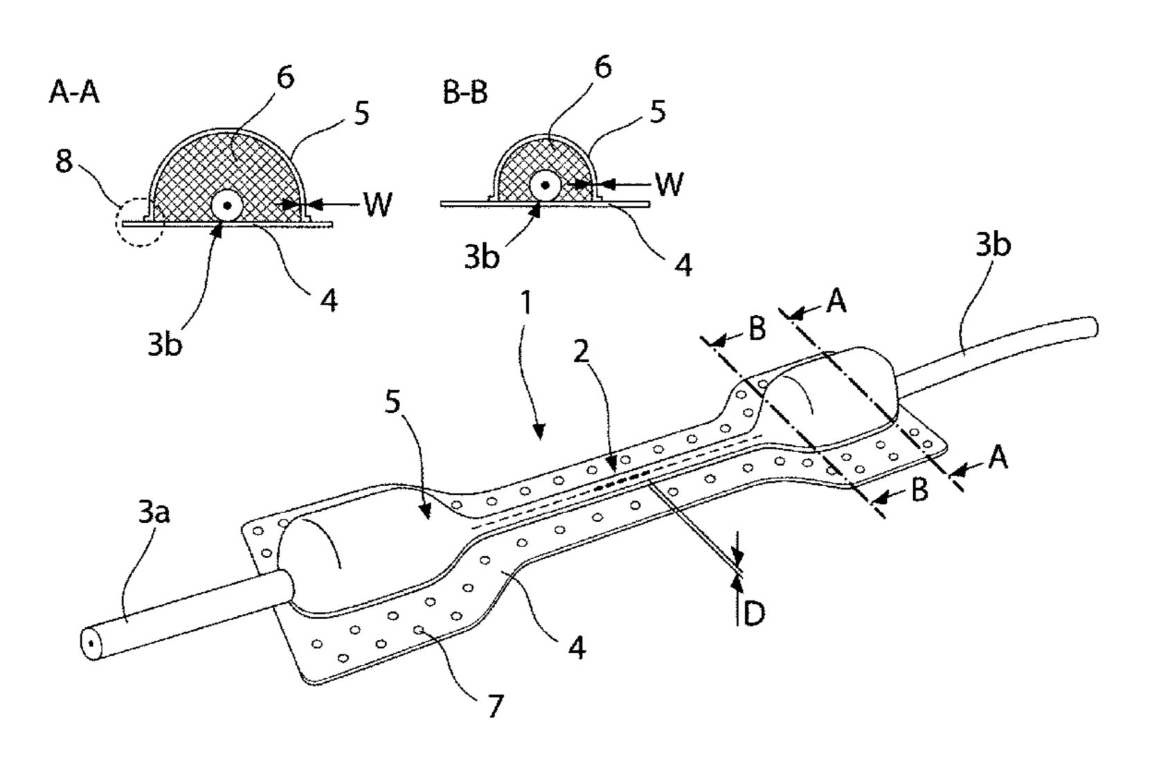
form a cavity underneath, with edges of the enlarged second part of the protective cover being bonded to the sensor carrier. Arranged in the cavity is an elastic filler which embeds the coupling points in a vibration damping manner. The protective cover with elastic filler accommodates thermal expansions and functions for dynamic measurements by the vibration damping.
