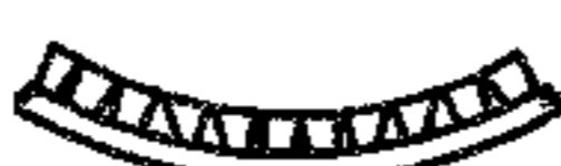
(iv) Cross-section of the substrate after re-crystallisation and growth up to the beginning of coalescence of the III-N layer at re-crystallisation temperature
