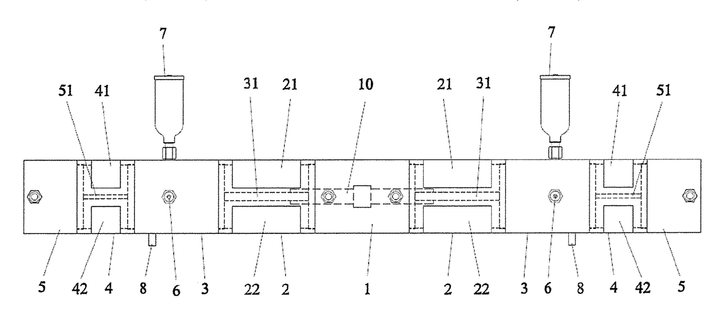
cylindrical homogenized main body is integrally connected with the long oil cylinder by virtue of one of the main connecting sleeves. Each high pressure cylindrical homogenized main body is integrally connected with the corresponding short oil cylinder by virtue of one of the auxiliary connecting sleeves.
