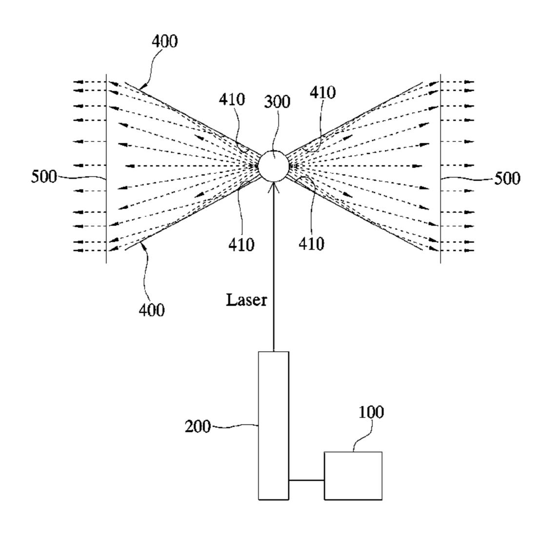
reflective structure has a reflective surface inclined in a direction away from the phosphor-containing emitter, wherein the reflective surfaces of the reflective structures are symmetrical with each other with respect to the phosphor-containing emitter. In accordance with the present disclosure, the lighthouse lantern may generate high output with low input power and thus has improved power efficiency, may suppress frequent failures near sea or seawater, and may reduce production costs.
