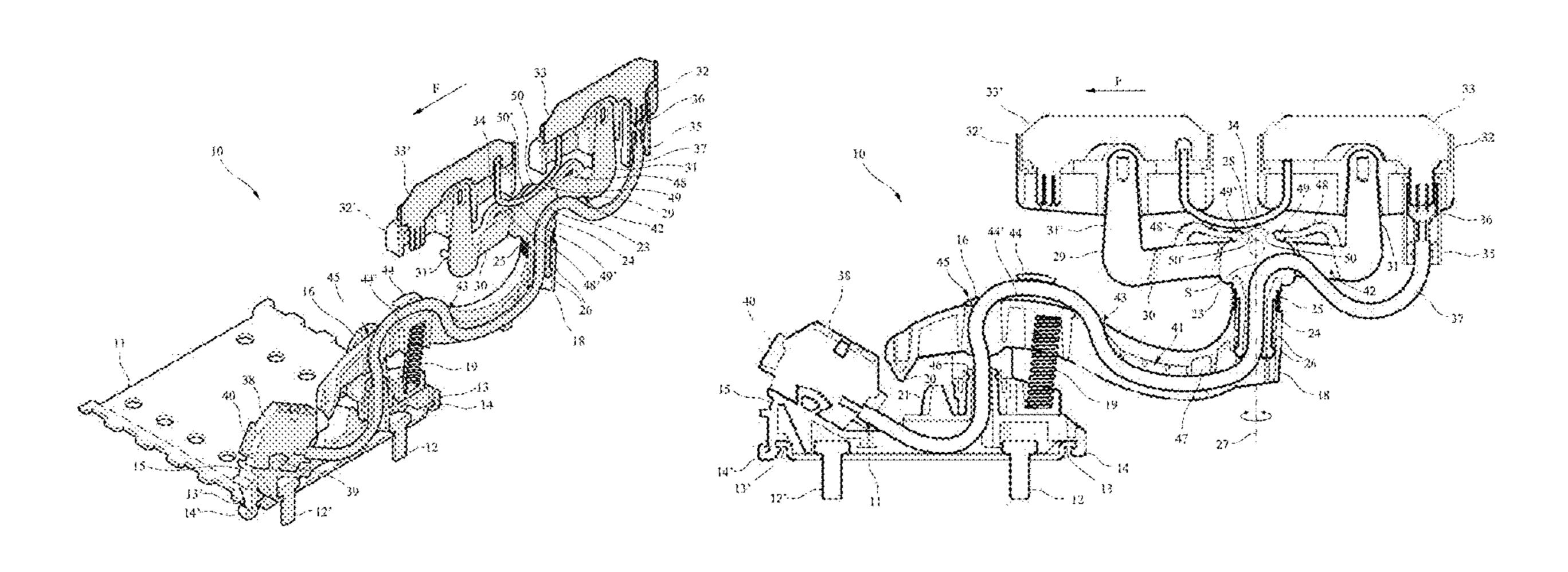
which connects the contact piece to a connection terminal for the electrical loads in an electrically conductive manner. A conductor line system includes a conductor line and at least one electrical load that can be moved on the conductor line in the longitudinal direction of the conductor line. The conductor line has at least one electrically conductive conductor strand for bringing into sliding contact with at least one contact piece of a current collector.
