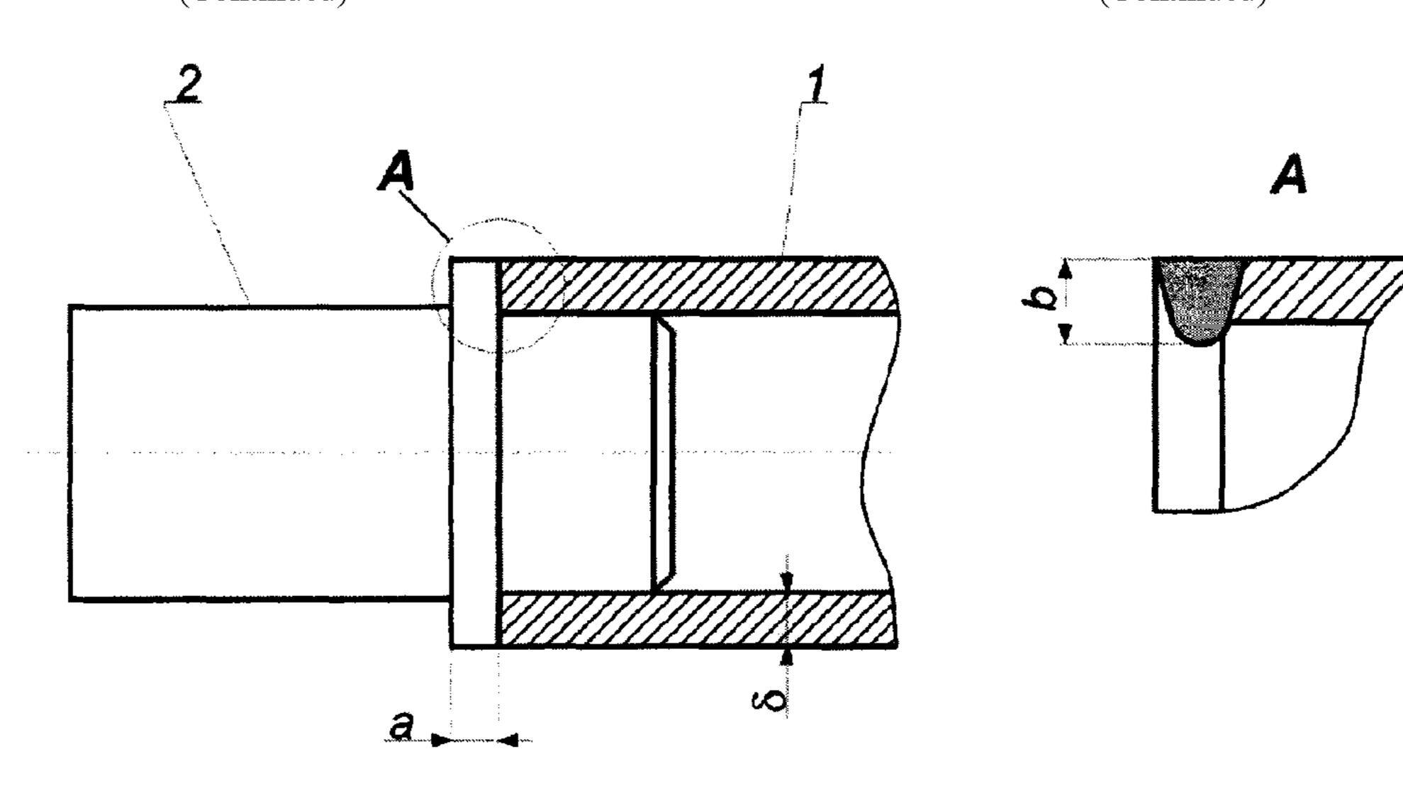
achieved through the formation of a ferrite phase in the metal of the seam by adjusting the structure of a joint between the casing and the plug of ferrite-martensite and ferrite steels in various combinations and by keeping the necessary ranges of the size ratios to ensure the formation of the aforesaid phase.
