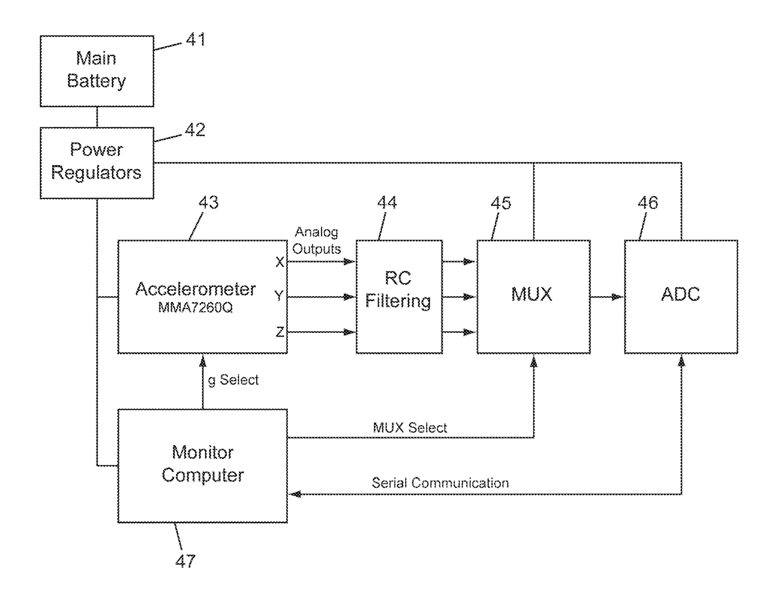
Figure 4: Belt Node Accelerometer
