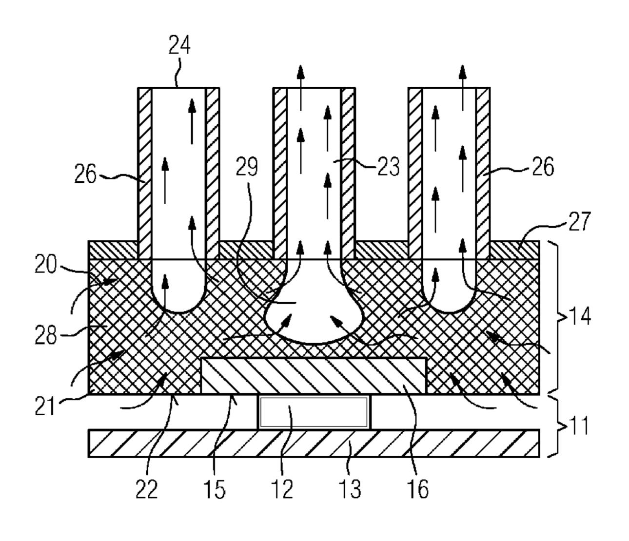
cooling chimney which lead from inlet openings in the upper side of the cooling member to the cooling chimney.
