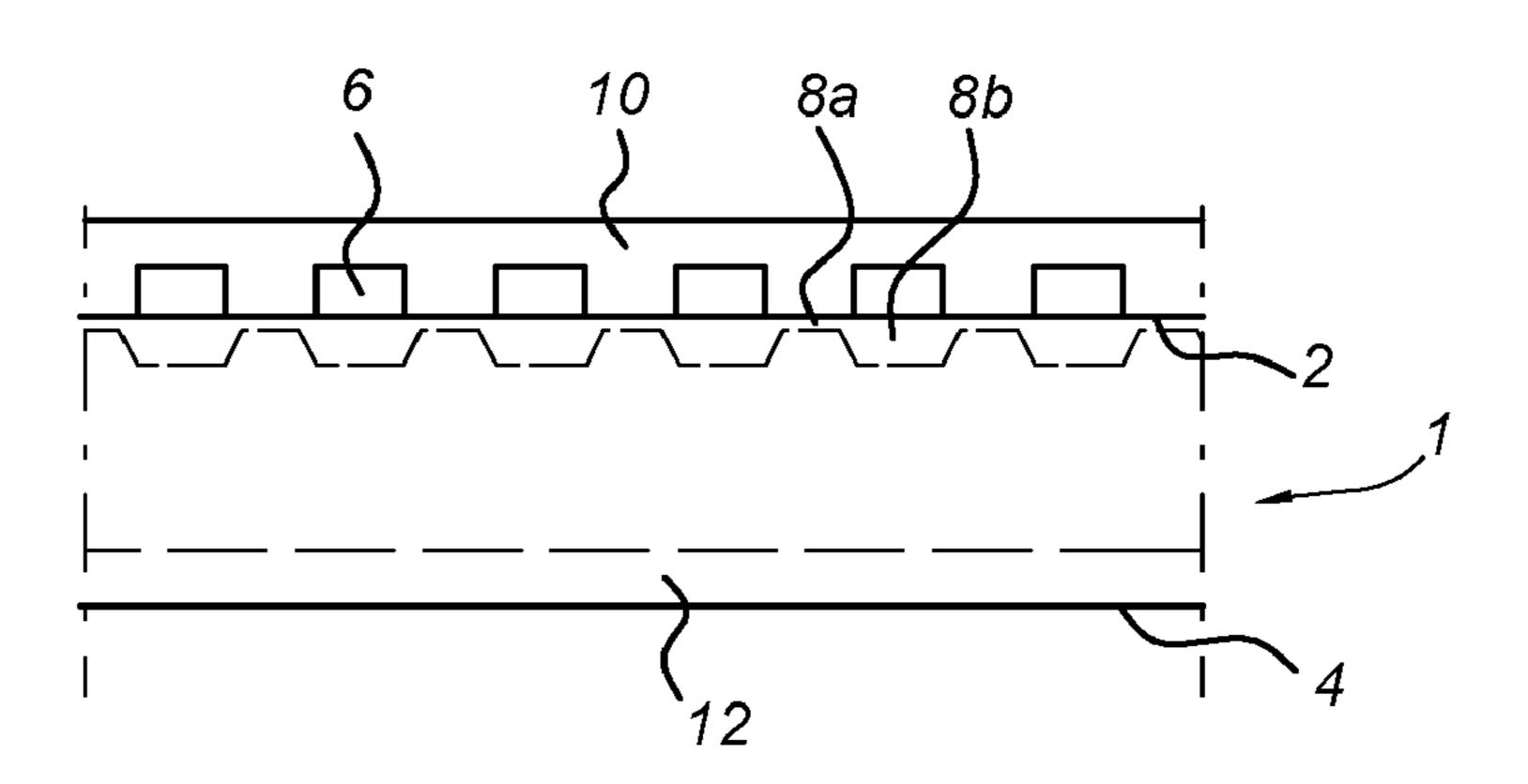
8a) through boron absorption by the undoped silicon oxide. The silicon oxide (10) acts as a boron absorber to obtain the desired concentration of the boron doped region (8).
