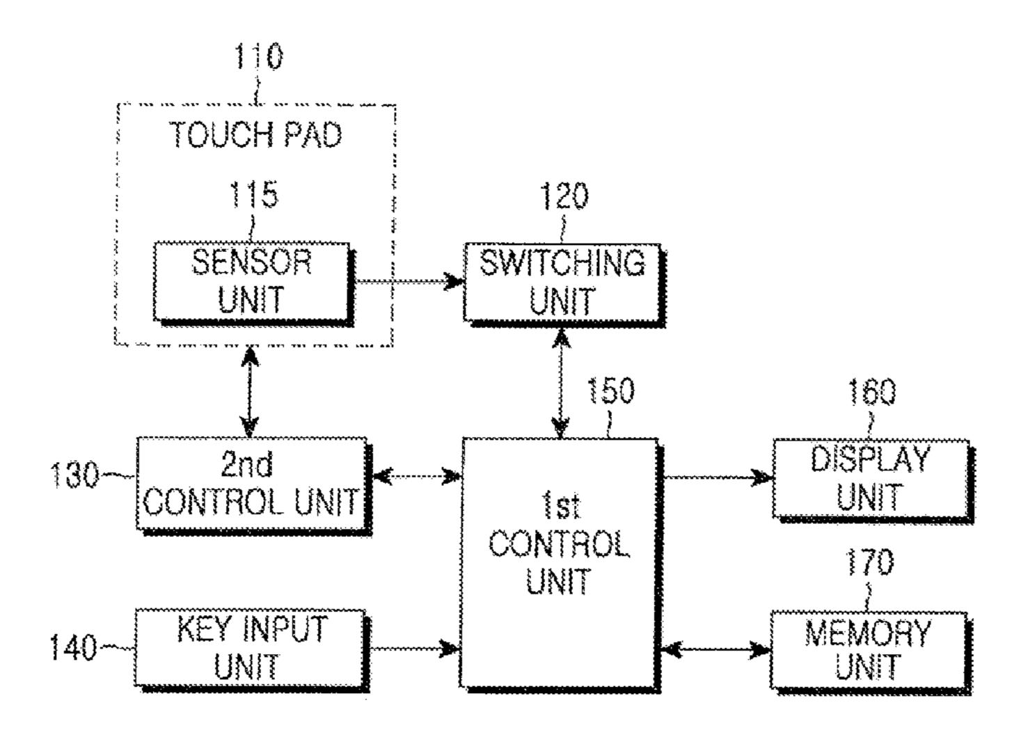
mode, the multimedia processor is activated when a user presses the touchpad, thereby making it possible to process signals input by touching the touchpad, particularly, to keep the user interface. Furthermore, the multimedia processor embedded in the portable terminal can reduce the consumption of battery power required to maintain the user interface, as compared with multimedia processors maintaining operating in a conventional polling method.
