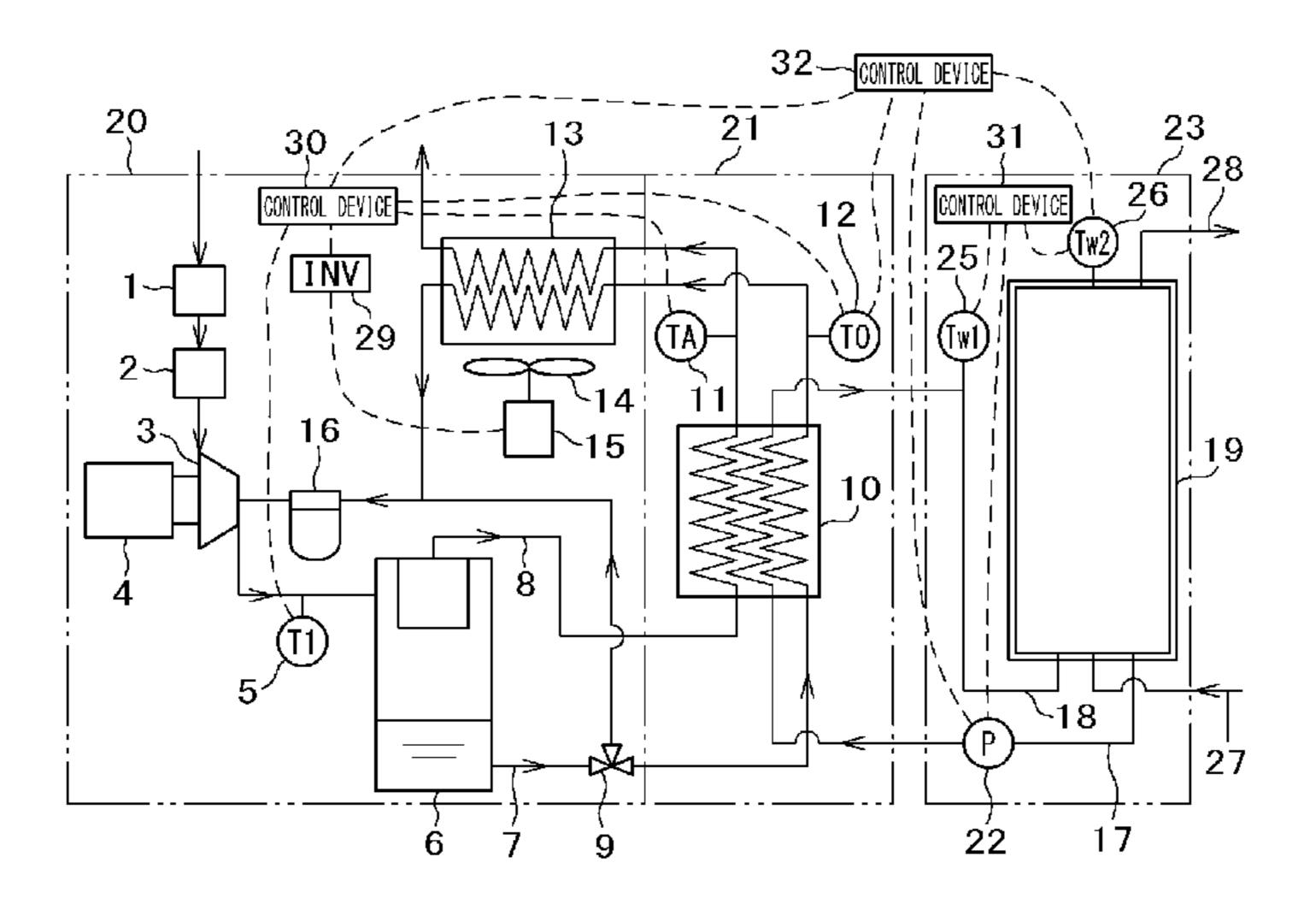
waste-heat recovery heat exchanger and the hot-water storage tank; a circulation pump (22) provided to these circulation circuits; and a control device (32) which, in cases when the temperature of the oil or the compressed gas subjected to heat exchange in the waste-heat-recovery heat exchanger is equal to or less than the temperature of the hot water in the hot-water storage tank, stops the circulation pump or reduces the rotational frequency of the circulation pump.
