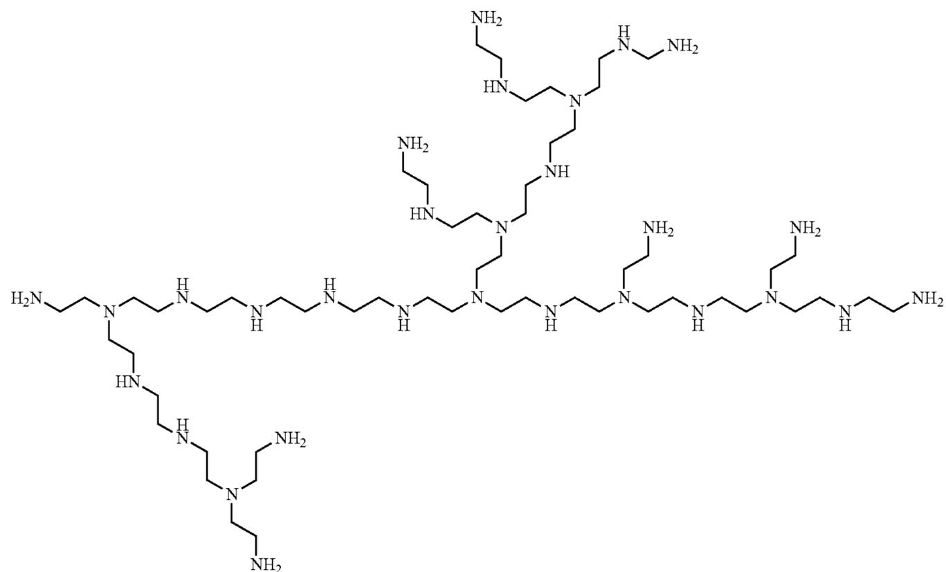
The unsubstituted initial polyethylenimine (PEI1) contained  $(2 \times 9) + (1 \times 13) = 31$  amine hydrogens on the primary and secondary nitrogen atoms. When reacted with 26 mol equivalents of propylene oxide,  $26/31 \times 100 = 83.9$  mol. % of the amine hydrogens of the primary and secondary nitrogen atoms have been replaced by a 2-hydroxypropyl group or a 1-hydroxypropane-2-yl group. In the structure of (PEI2), only 2-hydroxypropyl groups have been shown for the sake of simplicity.
