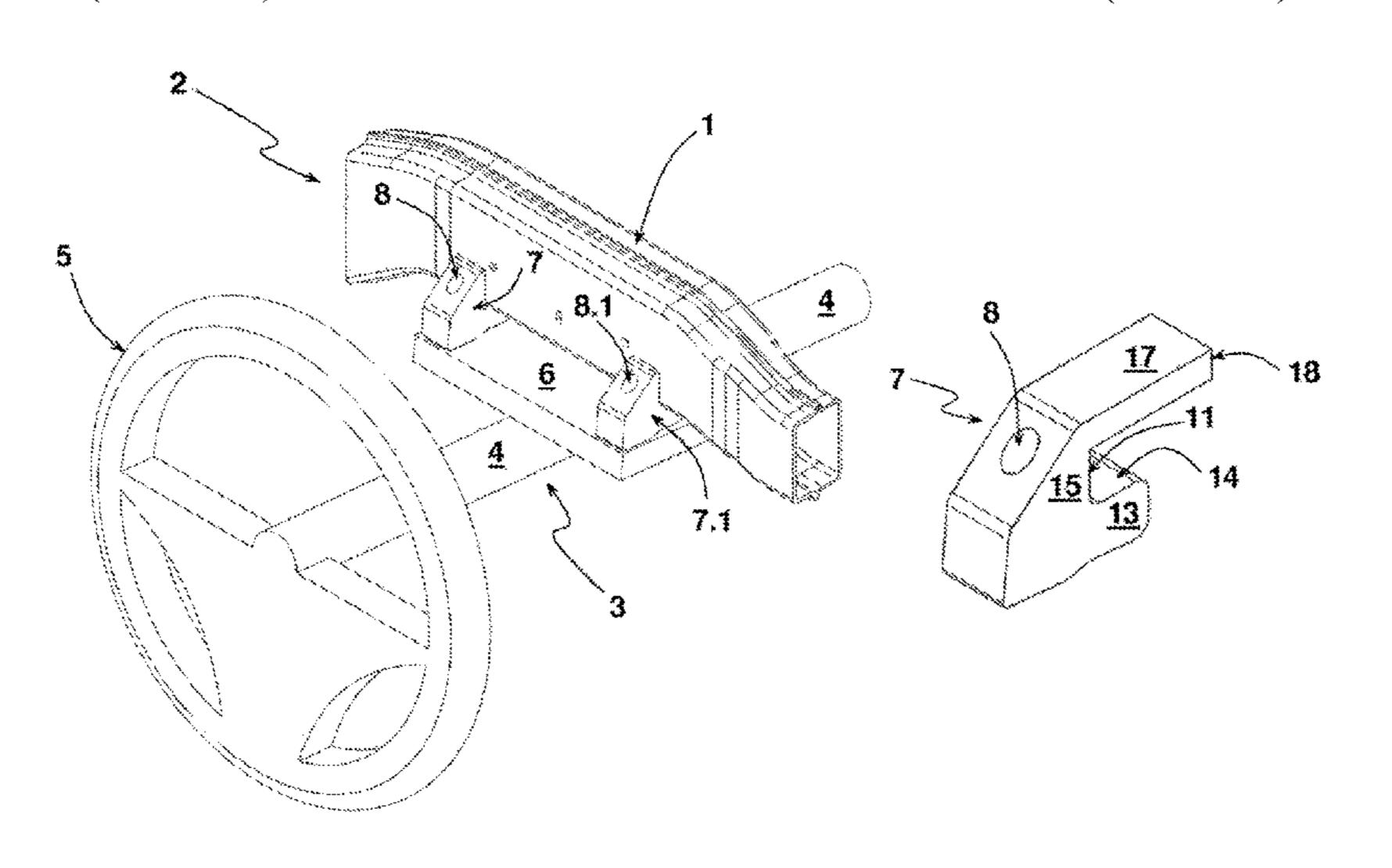
surface provided by a first limb at a first outer wall of the transverse carrier. The steering column holder has a further limb extending below the transverse carrier. The steering column holder carries a support projection which extends through the outer wall of the transverse carrier adjoining the support surface of the steering column holder and up to at least the opposite wall of the transverse carrier. The support projection is connected in a vibration-coupled manner to this opposite wall.
