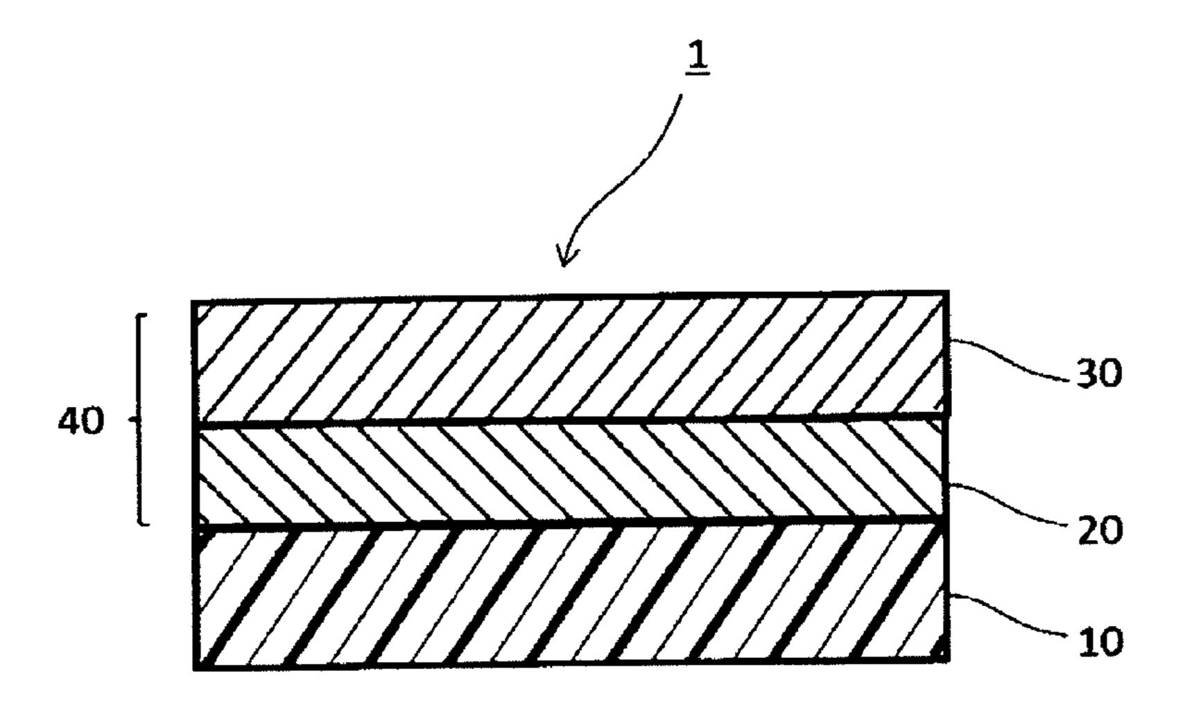
active ray-cured resin contains polyfunctional urethane (meth)acrylate as a polymerization component; and wherein the filler has a volume average particle size of 40 nm or less.
