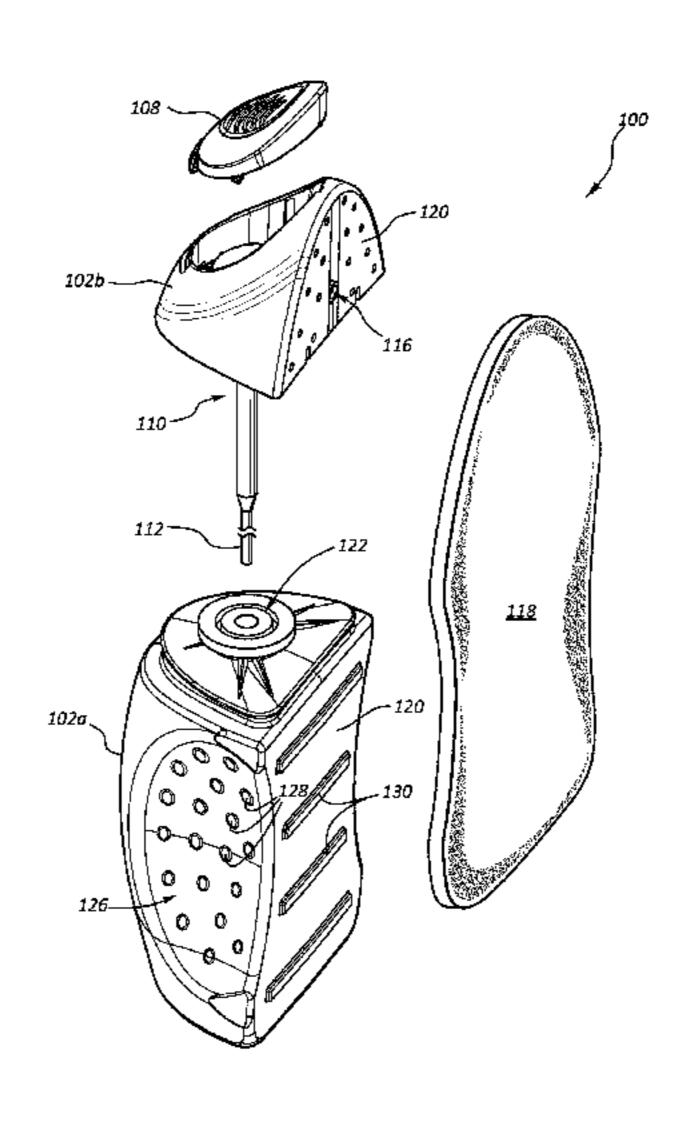
device may dispense a metered dose of composition, in a generally horizontal direction, onto and/or into a nonwoven or other substrate. The dispensing mechanism may not rely on gravity for dispensing, and may be sealed to prevent unwanted backflow of shower water or other material, preventing contamination.
