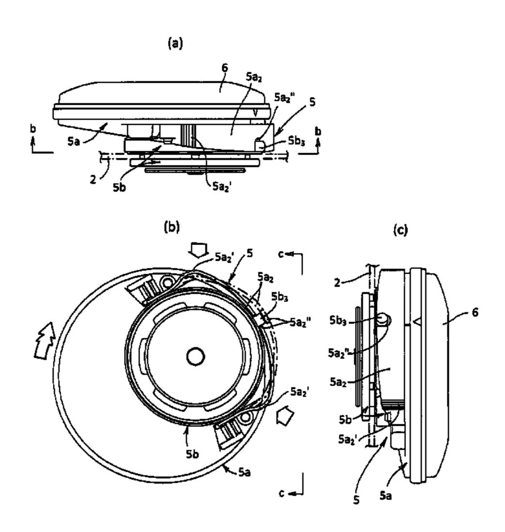
simultaneously when the filter is connected to the face piece, while unlocking motion of the lock mechanism precedes disconnecting motion of the bayonet connection mechanism so that unlocking of the connection precedes disconnection of the filter when the filter is disconnected from the face piece.
