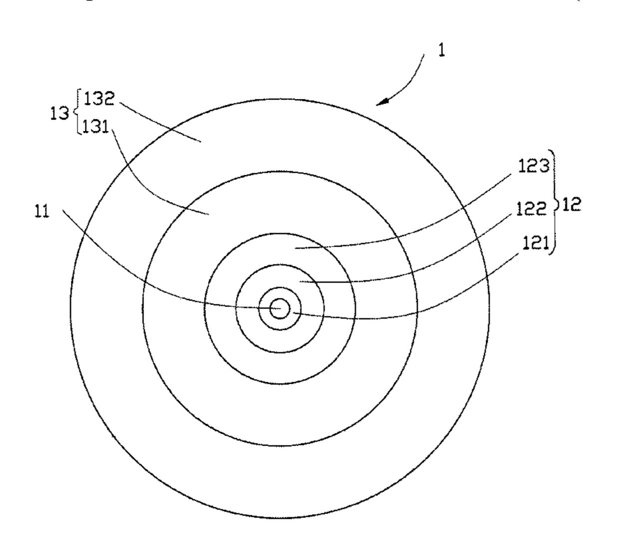
thickness, and the coating comprises an inner coating of 25 to 40  $\mu$ m thickness, and an outer coating of 25 to 35  $\mu$ m thickness and an ellipticity of less than 2%. The optical fiber has high durability and large effective transmission area, a method and system for preparing such optical fiber are also disclosed.
