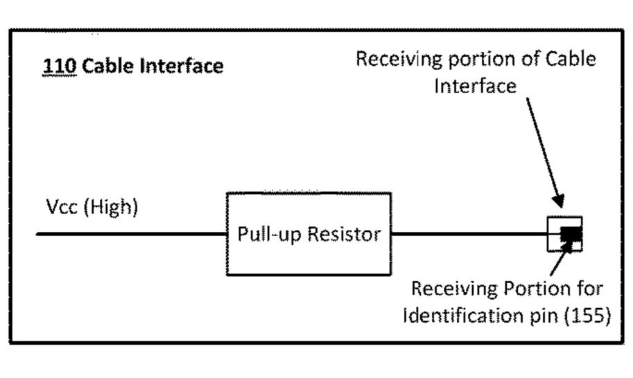
(1) When the cable is disconnected between the power converter 200 and the controller 73, the pull-up resistor pulls the receiving portion of the cable interface for an identification pin of cable 150 to a predetermined high output level, and the signal is tied to ground at the power converter 200
