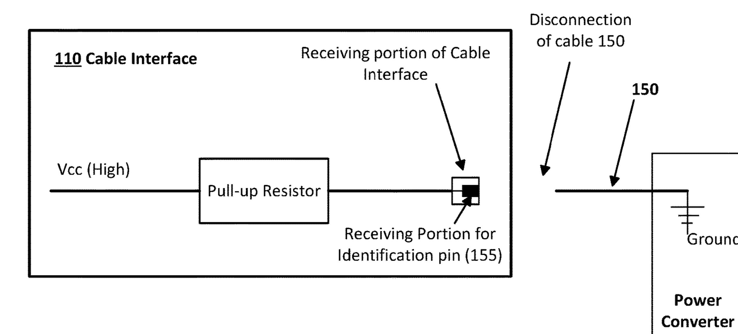
(1) When the cable is disconnected between the power converter 200 and the controller 73, the pull-up resistor pulls the receiving portion of the cable interface for an identification pin of cable 150 to a predetermined high output level, and the signal is tied to ground at the power converter 200
