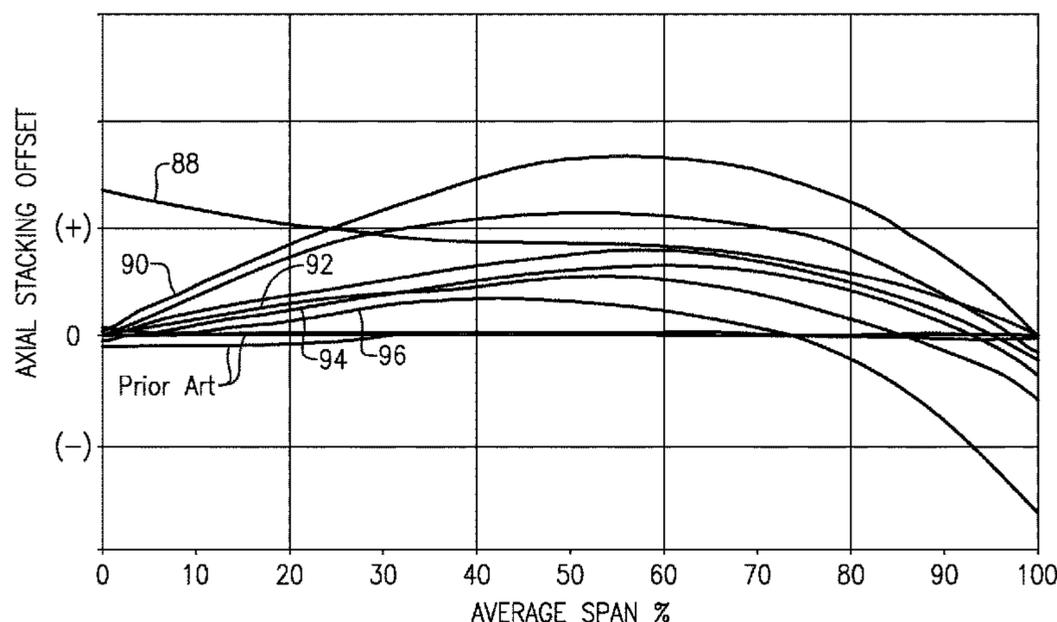
a negative slope from 90% span to 100% span. The negative slope leans forward relative to an engine axis.
