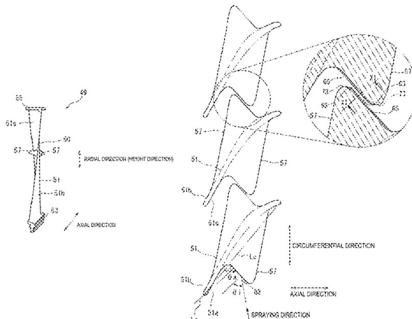
turbine rotor blade also includes a coating layer which is made of a Co-based alloy having a single composition on a surface of at least one of the first and second facing surfaces with a diffusion layer having a thickness of 10 μm or less provided between the coating layer and the surface.
